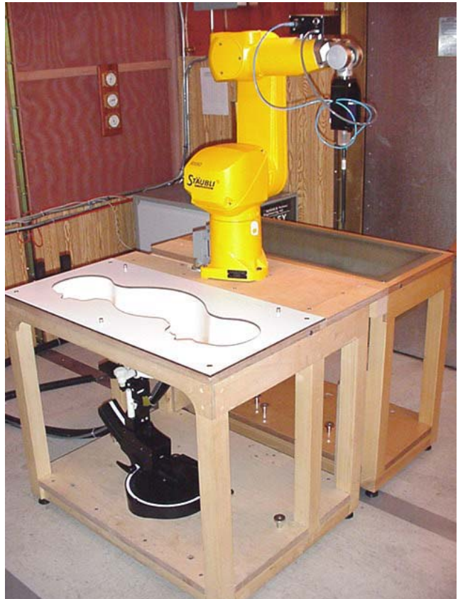
DASY4 SAR Measurement System with SAM phantom
