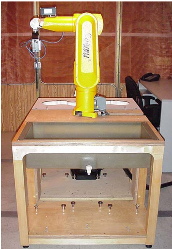
DASY4 SAR Measurement System with planar phantom
