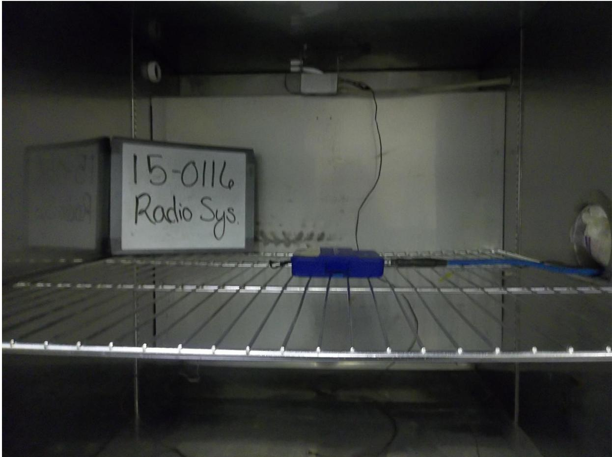
**Figure 6. Frequency Stability Test Setup**
