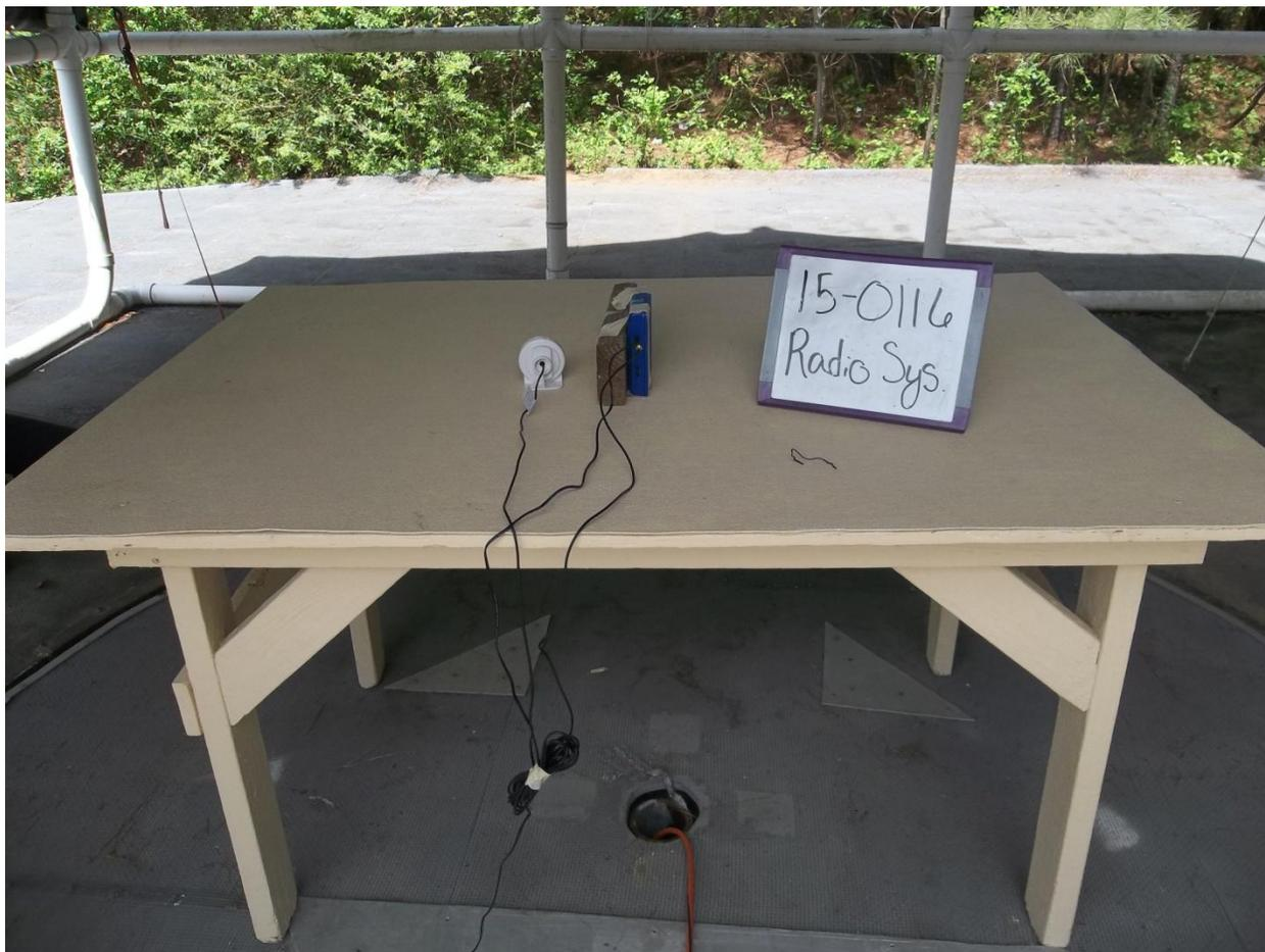
**Figure 1. Radiated Emissions Test Setup, Front (Radio Test with EUT in worst case position)**
