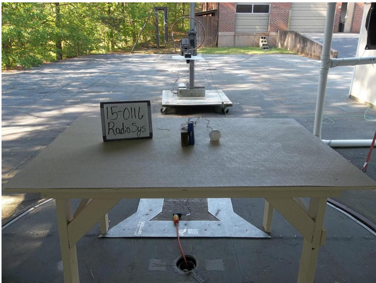
**Figure 2. Radiated Emissions Test Setup, Rear 9 kHz to 30 MHz (Normal Operation with EUT in worst case position)**
