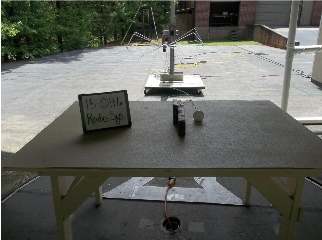
**Figure 3. Radiated Emissions Test Setup, Rear 30 MHz to 200 MHz (Radio Test with EUT in worst case position)**
