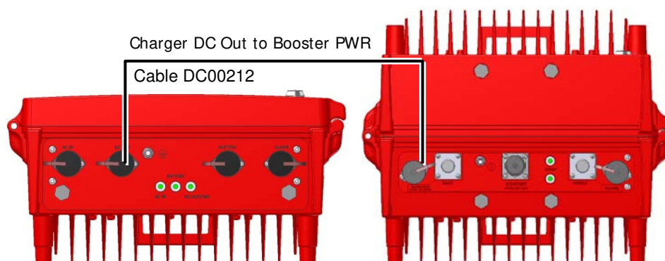
Figure 3-19 Battery Charger to Booster Power Connections
