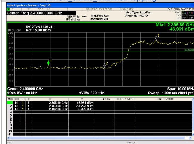
Out Of Band Emission(Left) 8DPSK_3-DH5_Channel Hopping
