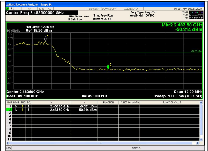
Out Of Band Emission(Right) \pi/4 DQPSK_2-DH5_Channel Hopping
