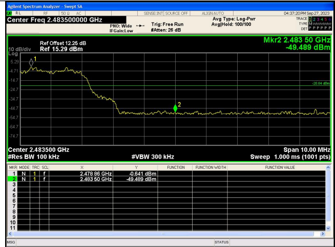
Out Of Band Emission(Right) 8DPSK_3-DH5_Channel Hopping
