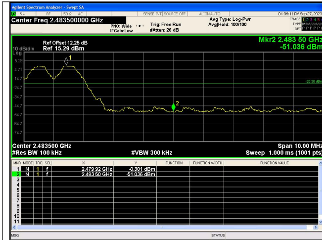
Out Of Band Emission(Right) GFSK_DH5_Channel Hopping
