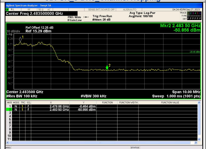
Out Of Band Emission(Right) 8DPSK_3-DH5_Channel Hopping
