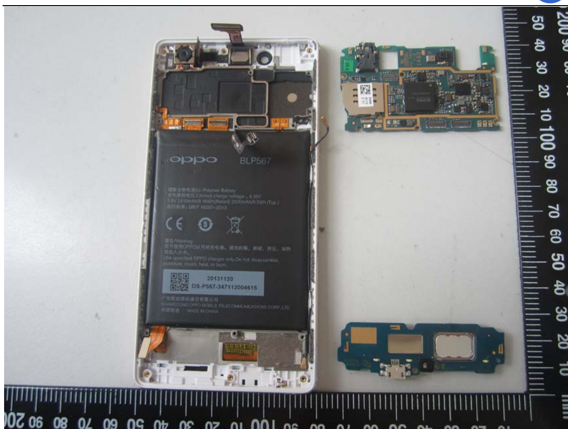
2. Mainboard front view with shielding
