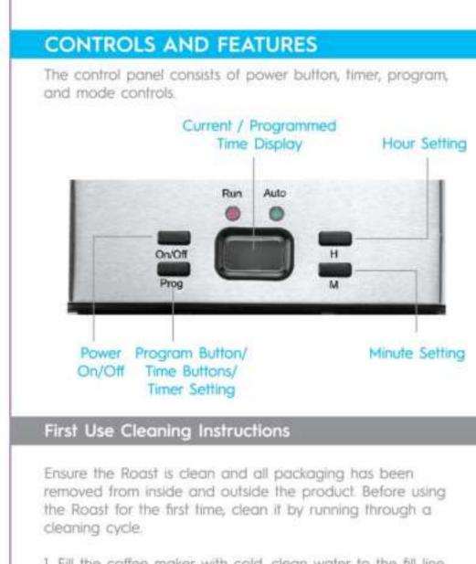
1. Fill the coffee maker with cold, clean water to the fill line. Place the filter into the machine (without adding coffee), and close the lid.
