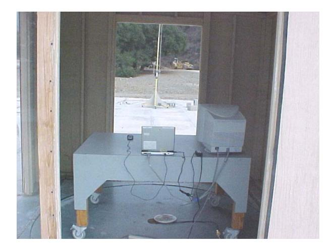
Radiated Emissions Measurement (30-1000 MHz) (Rear View) Setup
