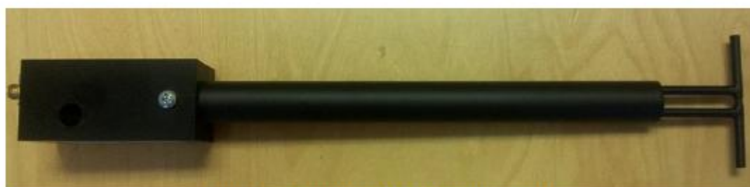
Figure 1 – MVG COMOSAR Validation Dipole
