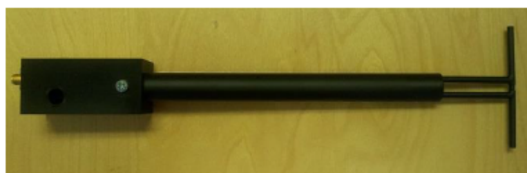
Figure 1 – MVG COMOSAR Validation Dipole
