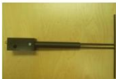
Figure 1 – MVG COMOSAR Validation Dipole
