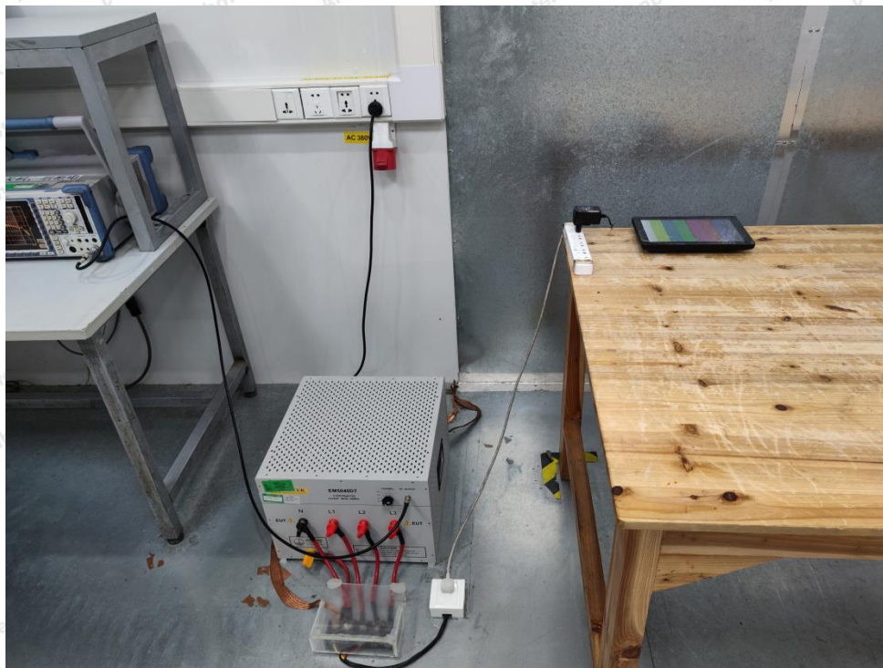
Photo of Conducted Emission Measurement
