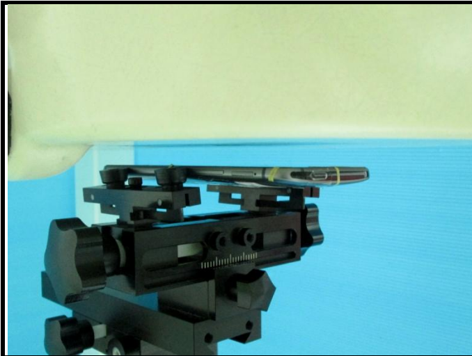
Front Face of EUT with 1.0 cm Gap
