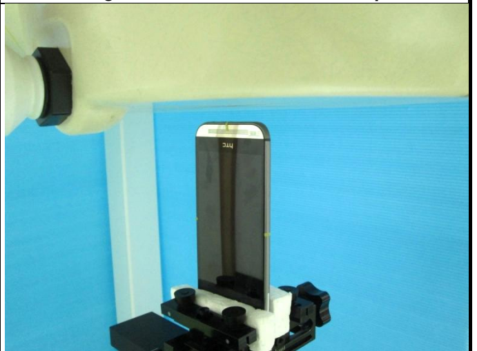
Bottom Side of EUT with 1.0 cm Gap
