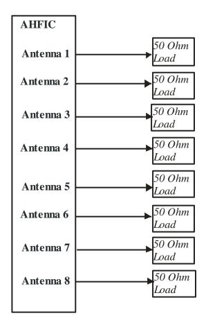
Based on antenna port conducted spurious emissions tests results, preliminary scans for radiated spurious emissions were performed in 30MHz – 22GHz frequency range. Two test configurations are needed for radiated spurious emission measurements. The first test is with PCS and AWS carriers operating at 40W/carrier. The second test is with the PCS carriers operating at 20W/carrier and the AWS carriers operating at 60W/carrier.
