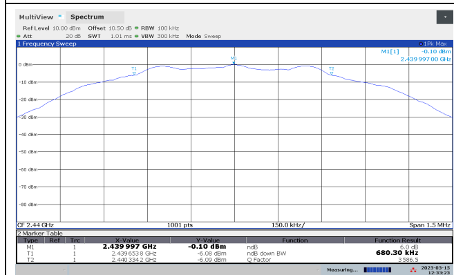
DTS BW, 2440 MHz, 1M
