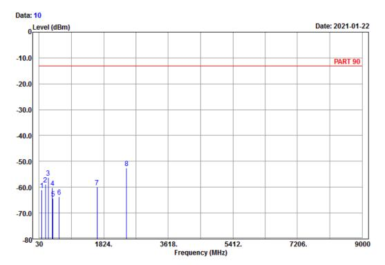
Site : 966 chamber 1 Condition: PART 90 Vertical Remark : LTE\_Band 26\_Link\_M-Ch
