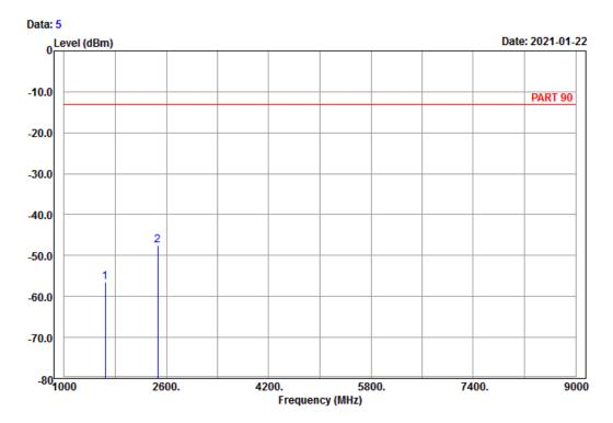
Site : 966 chamber 1 Condition: PART 90 Horizontal Remark : LTE\_Band 26\_Link\_H-Ch
