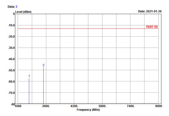
Site : 966 chamber 1 Condition: PART 90 Horizontal Remark : LTE\_Band 26\_Link\_M-Ch
