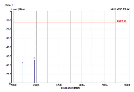
Site : 966 chamber 1 Condition: PART 90 Vertical Remark : LTE\_Band 26\_Link\_H-Ch
