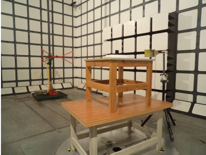
Radiated Emissions Test View (Below 1 GHz)
