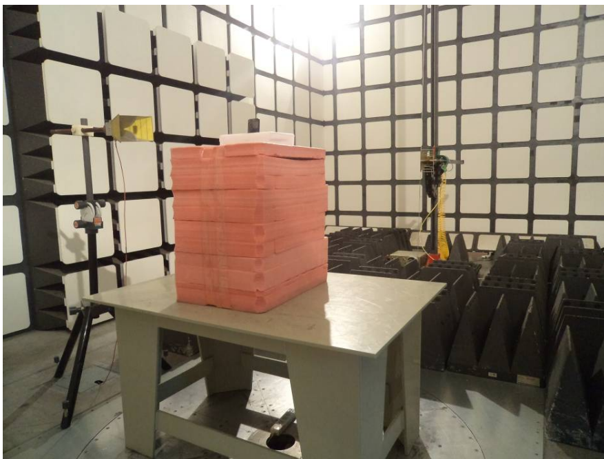
Radiated Emissions Test View (Above 1 GHz)
