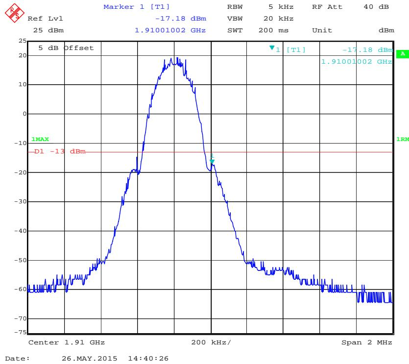
**PCS Band, Left Band Edge for GSM (8PSK) Mode**
