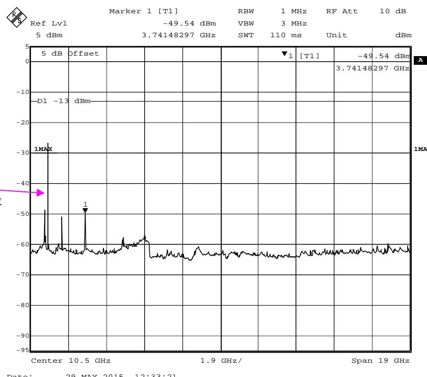
Fundamental test with notch filter
