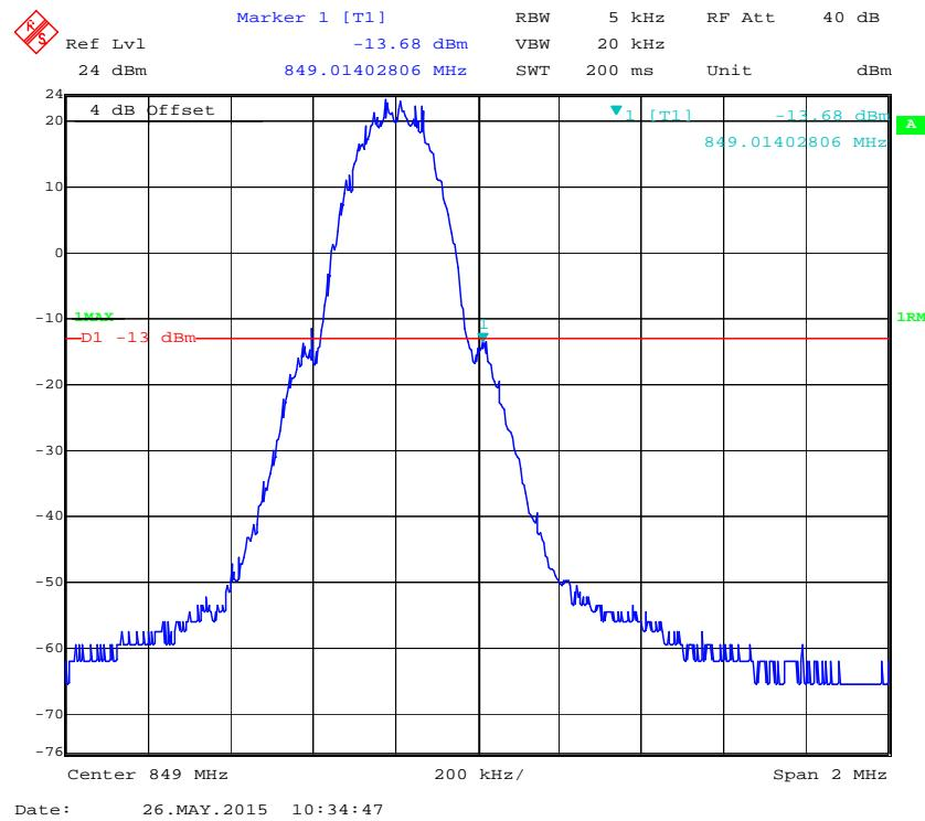
**Cellular Band, Left Band Edge for GSM (8PSK) Mode**
