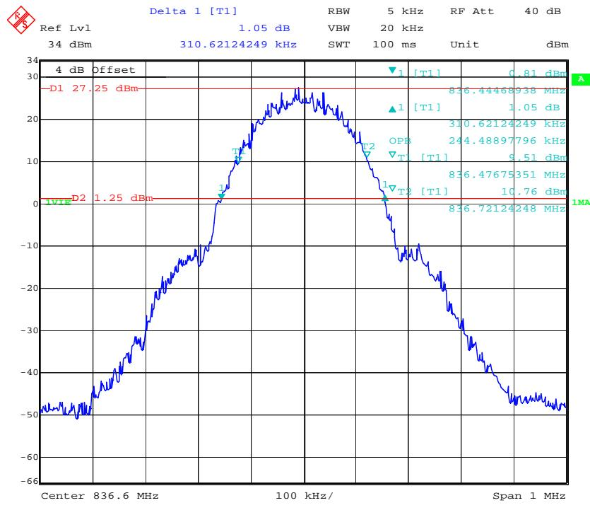
**99% Occupied &26 dB Emissions Bandwidth for GSM (8PSK) Mode**
