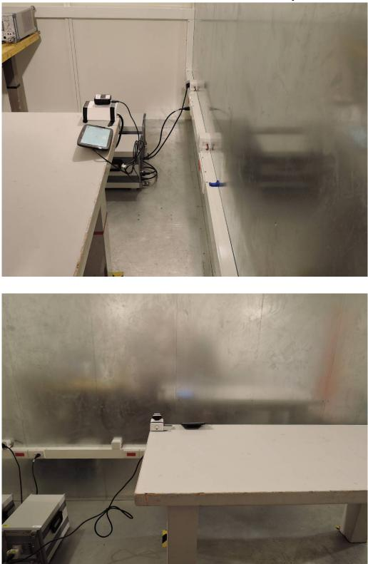
**AC Power-line Conducted Emission Set up Photo**
