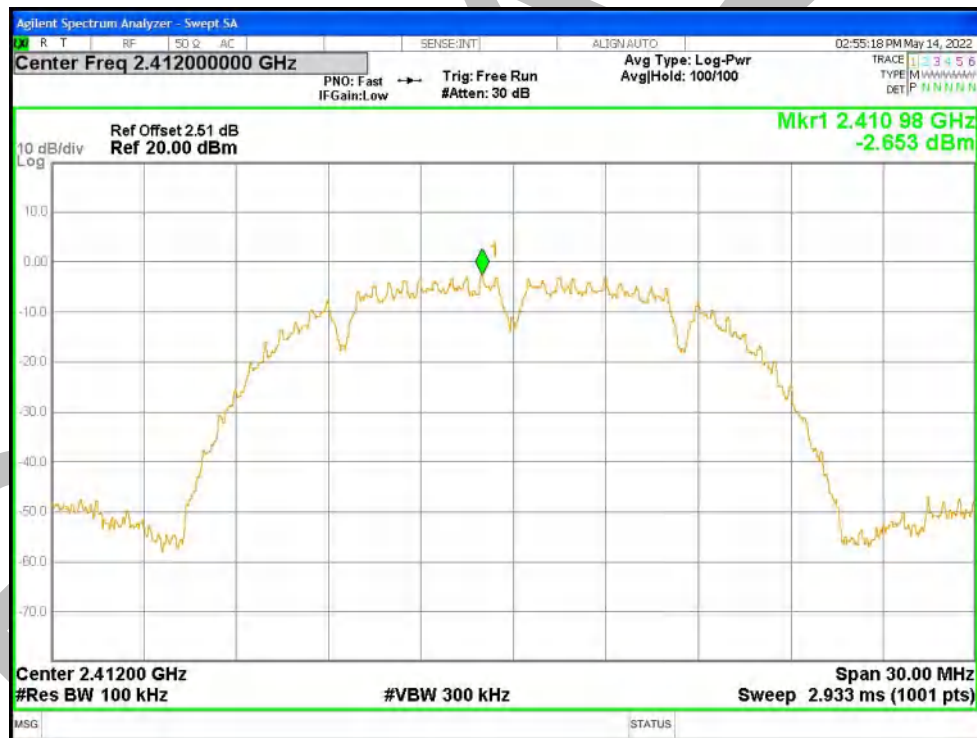
Tx. Spurious NVNT b 2412MHz Ant1 Emission
