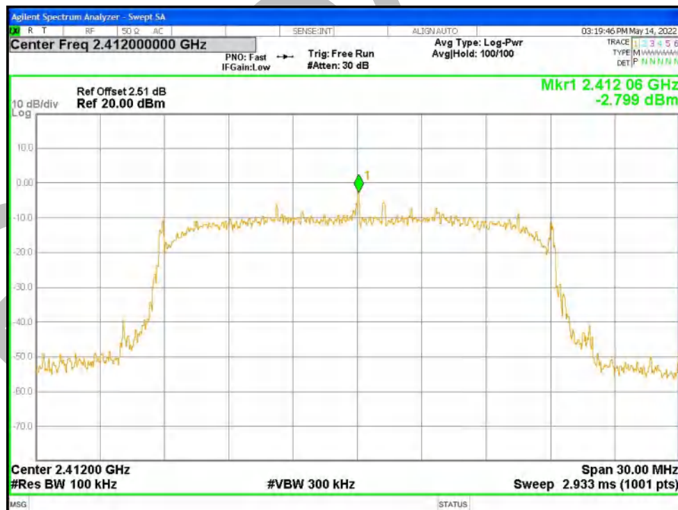
Tx. Spurious NVNT n20 2412MHz Ant1 Emission
