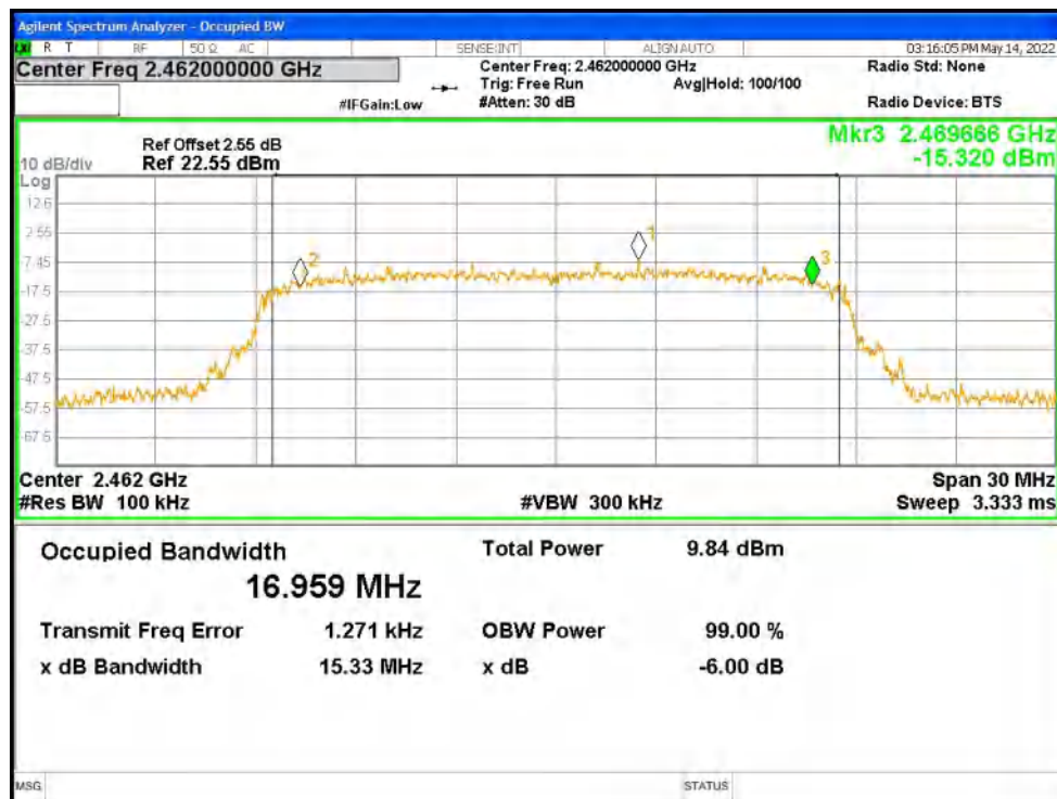
-6dB Bandwidth NVNT n20 2412MHz Ant1
