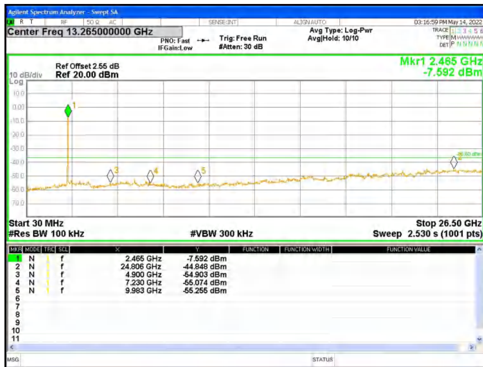
Tx. Spurious NVNT n20 2412MHz Ant1 Ref
