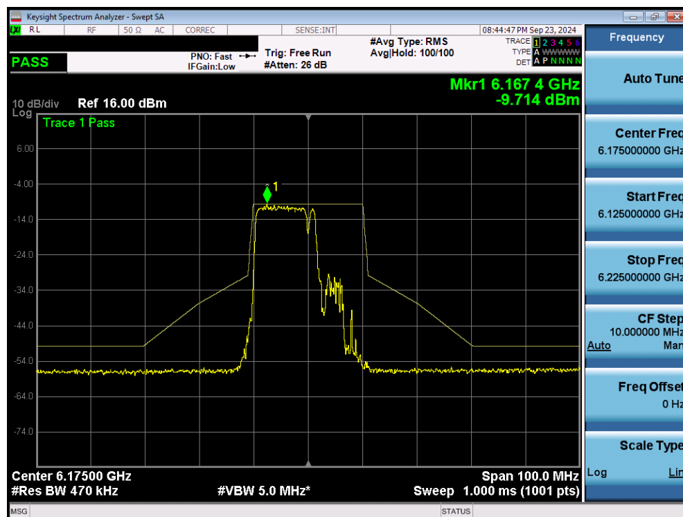
Plot 7-83. In Band Emissions Plot MIMO ANT2 (20MHz 802.11be (106+26 Tones) (UNII Band 5) – Ch. 45) - VLP
