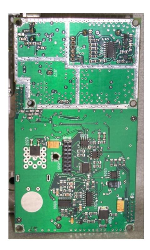
Photo 12. EUT, Top View of High Level Power Amplifier Board
