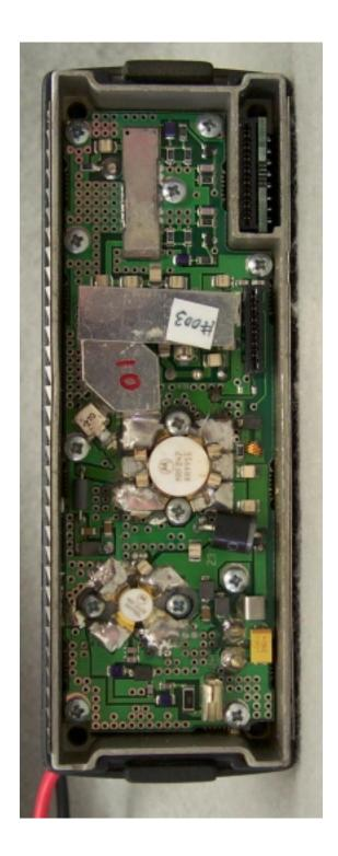
Photo 13. EUT, Bottom View of High Level Power Amplifier Board
