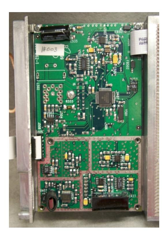
Photo 10. EUT, Top View of System Board with Shield Removed
