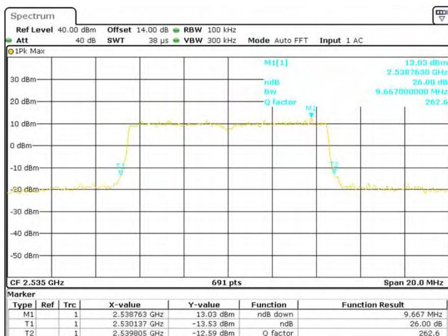
**QPSK (15.0 MHz) - 26 dB Bandwidth, Middle channel**
