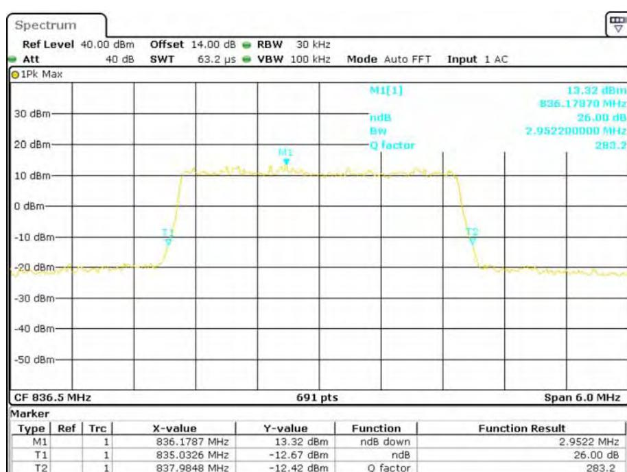
**QPSK (5.0 MHz) - 26 dB Bandwidth, Middle channel**
