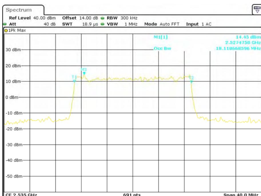
**QPSK (5.0 MHz) - 26 dB Bandwidth, Middle channel**
