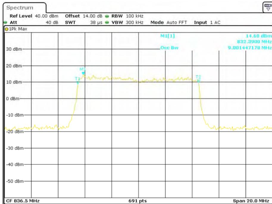
**16-QAM (10.0 MHz) - 99% Occupied Bandwidth, Middle channel**
