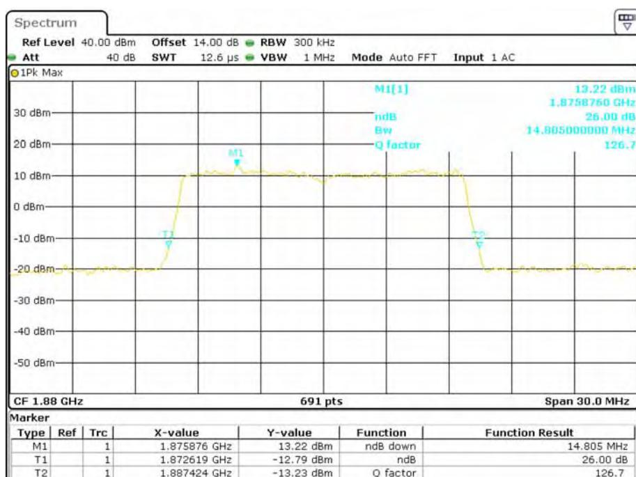
**QPSK (20.0 MHz) - 26 dB Bandwidth, Middle channel**
