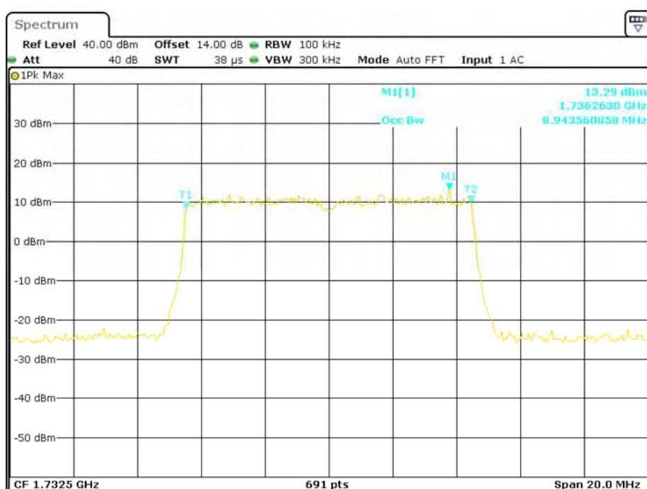
**QPSK (15.0 MHz) - 99% Occupied Bandwidth, Middle channel**
