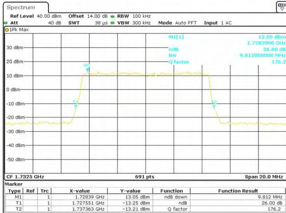
**16-QAM (10.0 MHz) - 26 dB Bandwidth, Middle channel**
