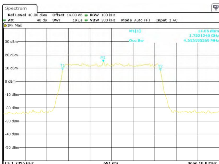
**QPSK (10.0 MHz) - 99% Occupied Bandwidth, Middle channel**
