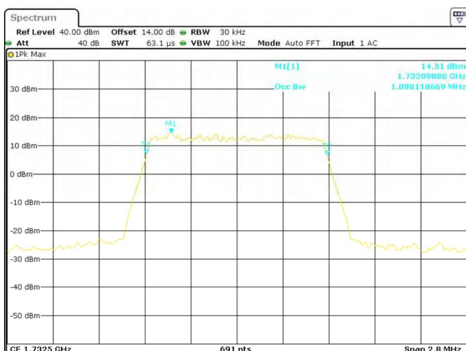
**QPSK (3.0 MHz) - 99% Occupied Bandwidth, Middle channel**
