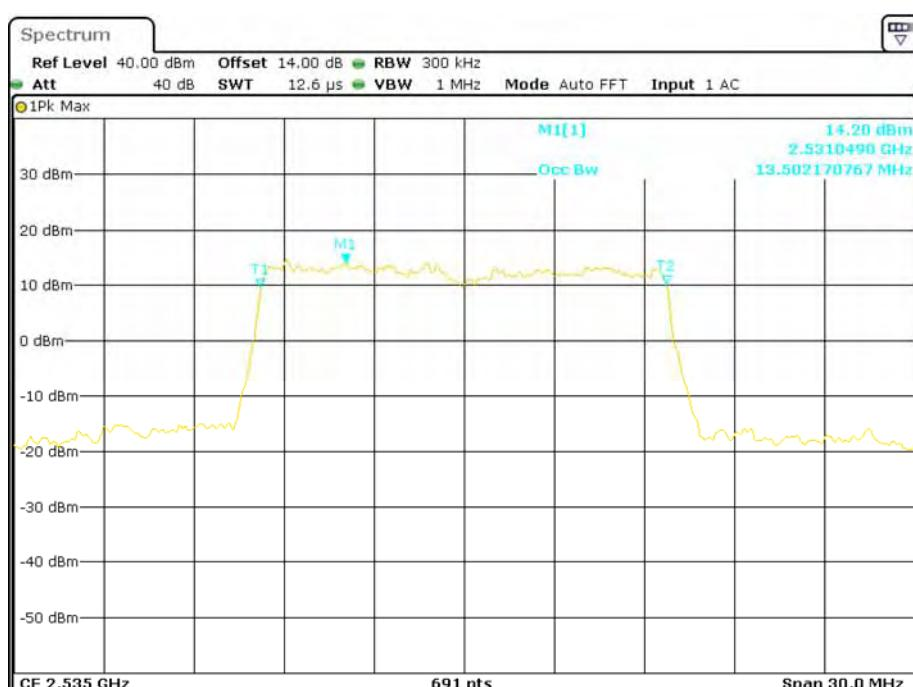
**QPSK (20.0 MHz) - 99% Occupied Bandwidth, Middle channel**
