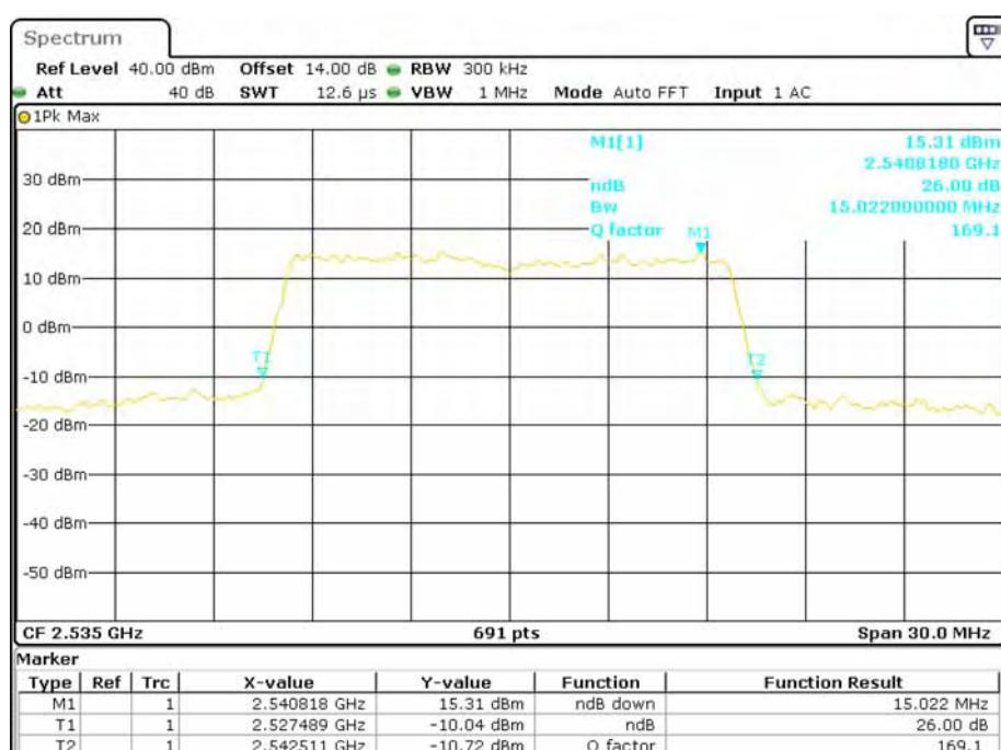
**QPSK (20.0 MHz) - 26 dB Bandwidth, Middle channel**
