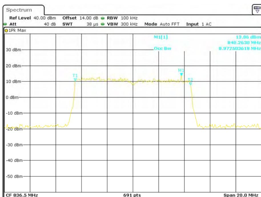
**QPSK (1.4 MHz) - 26 dB Bandwidth, Middle channel**
