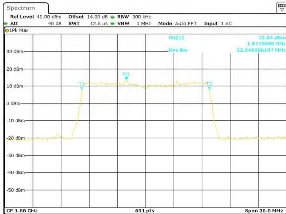
**16-QAM (15.0 MHz) - 99% Occupied Bandwidth, Middle channel**
