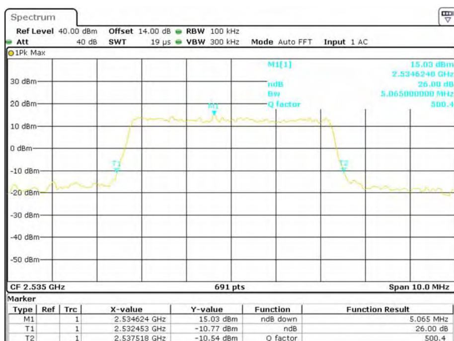
**QPSK (10.0 MHz) - 26 dB Bandwidth, Middle channel**
