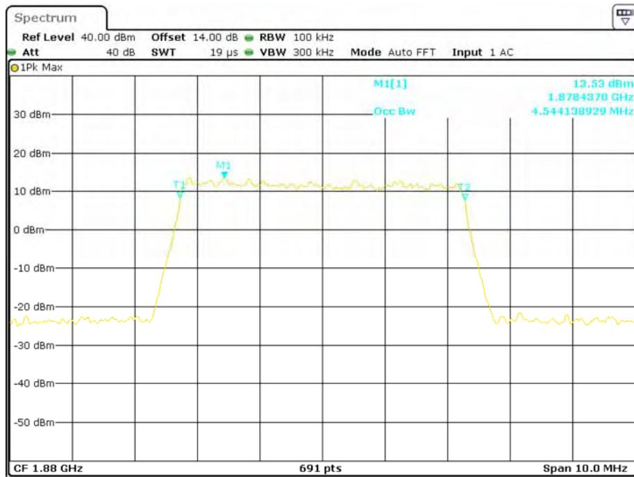
**16-QAM (5.0 MHz) - 99% Occupied Bandwidth, Middle channel**
