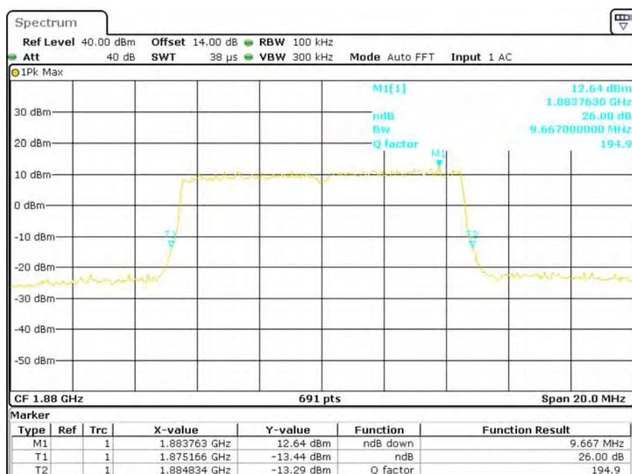
**QPSK (15.0 MHz) - 26 dB Bandwidth, Middle channel**
