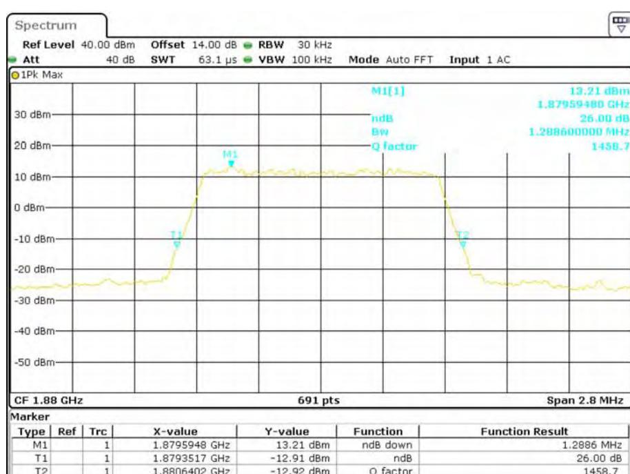
**QPSK (3.0 MHz) - 26 dB Bandwidth, Middle channel**
