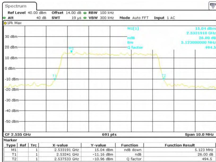
**16-QAM (5.0 MHz) - 26 dB Bandwidth, Middle channel**
