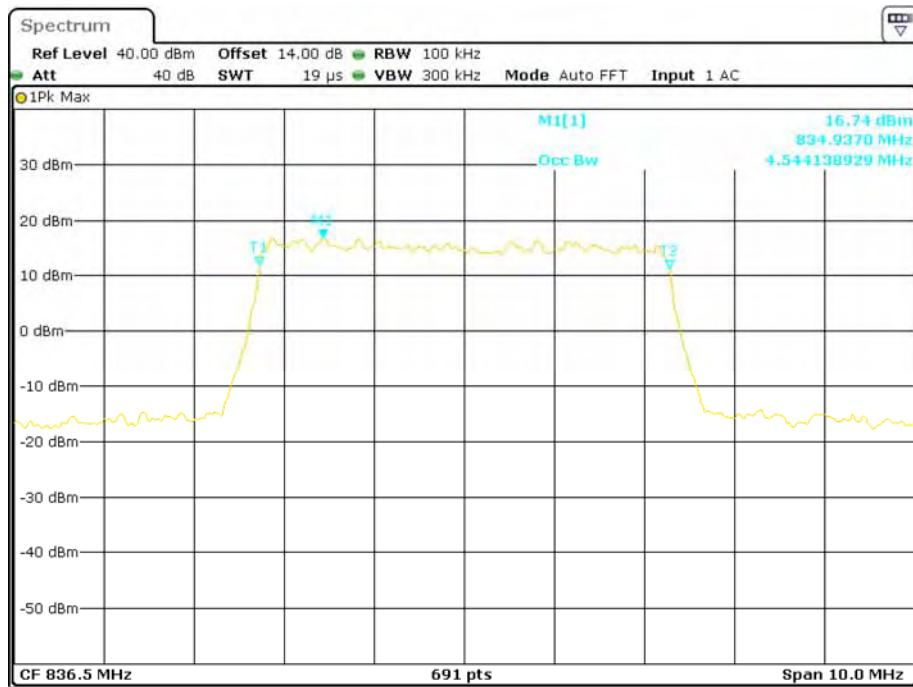
**16-QAM (5.0 MHz) - 99% Occupied Bandwidth, Middle channel**
