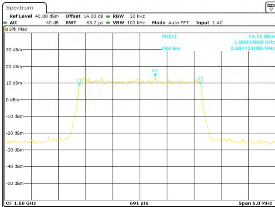
**16-QAM (3.0 MHz) - 99% Occupied Bandwidth, Middle channel**
