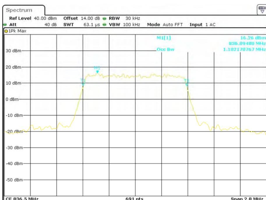
**QPSK (3.0 MHz) - 99% Occupied Bandwidth, Middle channel**
