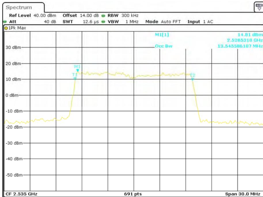
**16-QAM (15.0 MHz) - 99% Occupied Bandwidth, Middle channel**
