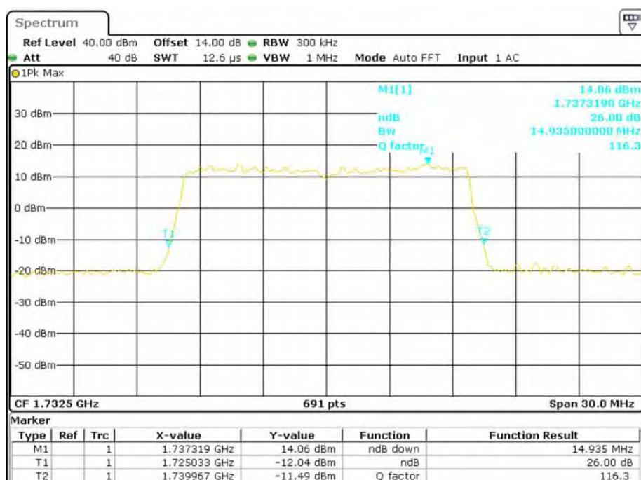
**QPSK (20.0 MHz) - 26 dB Bandwidth, Middle channel**
