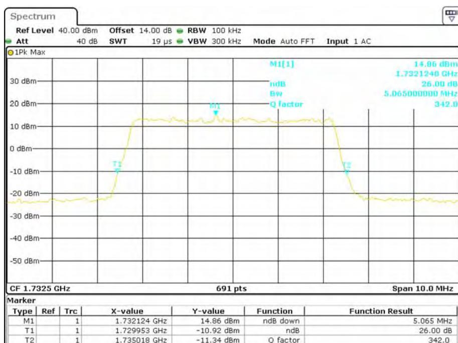
**QPSK (10.0 MHz) - 26 dB Bandwidth, Middle channel**
