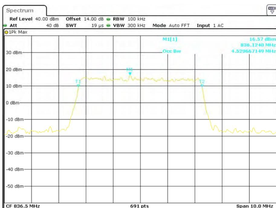
**QPSK (10.0 MHz) - 99% Occupied Bandwidth, Middle channel**
