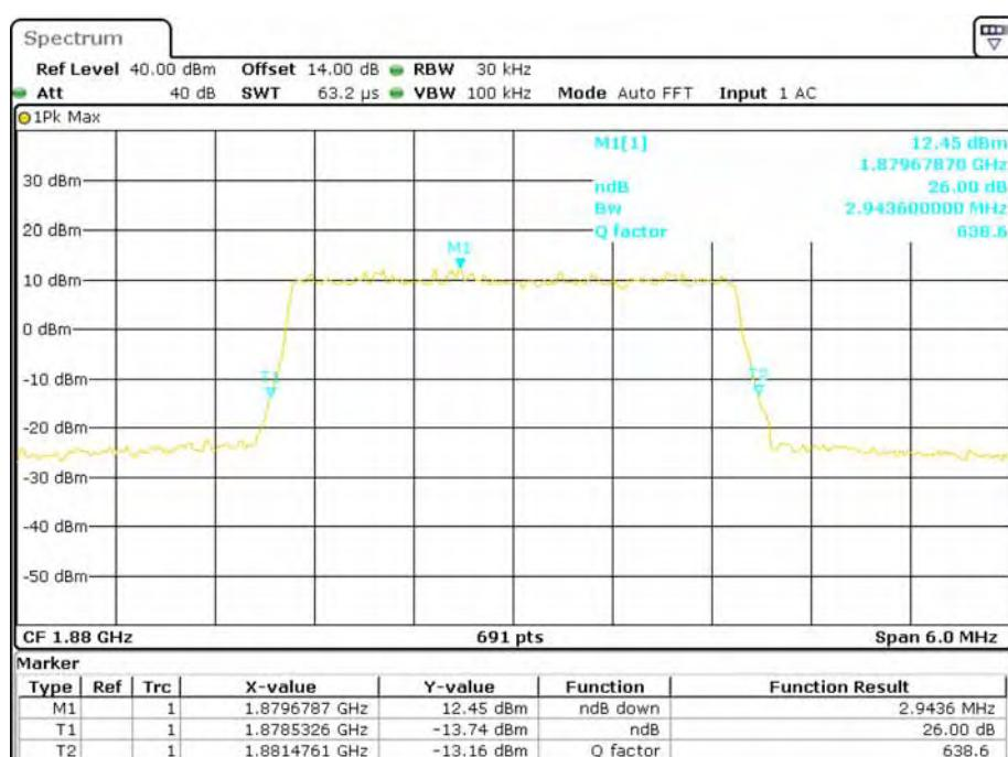
**QPSK (5.0 MHz) - 26 dB Bandwidth, Middle channel**
