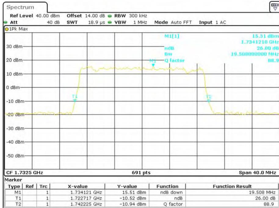
**16-QAM (20.0 MHz) - 26 dB Bandwidth, Middle channel**
