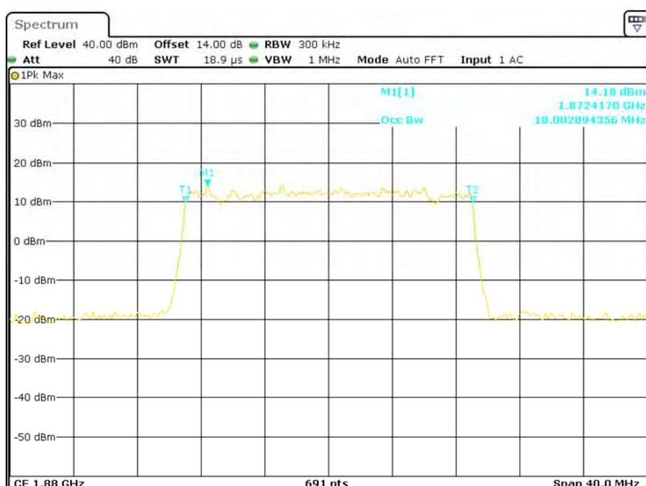
**QPSK (1.4 MHz) - 26 dB Bandwidth, Middle channel**
