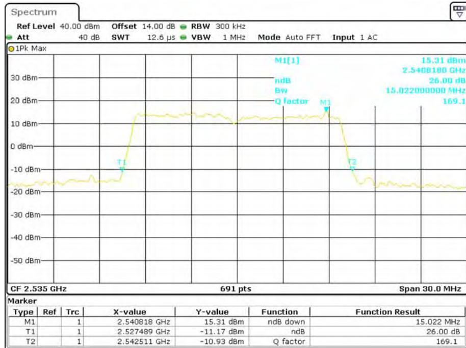
**16-QAM (15.0 MHz) - 26 dB Bandwidth, Middle channel**
