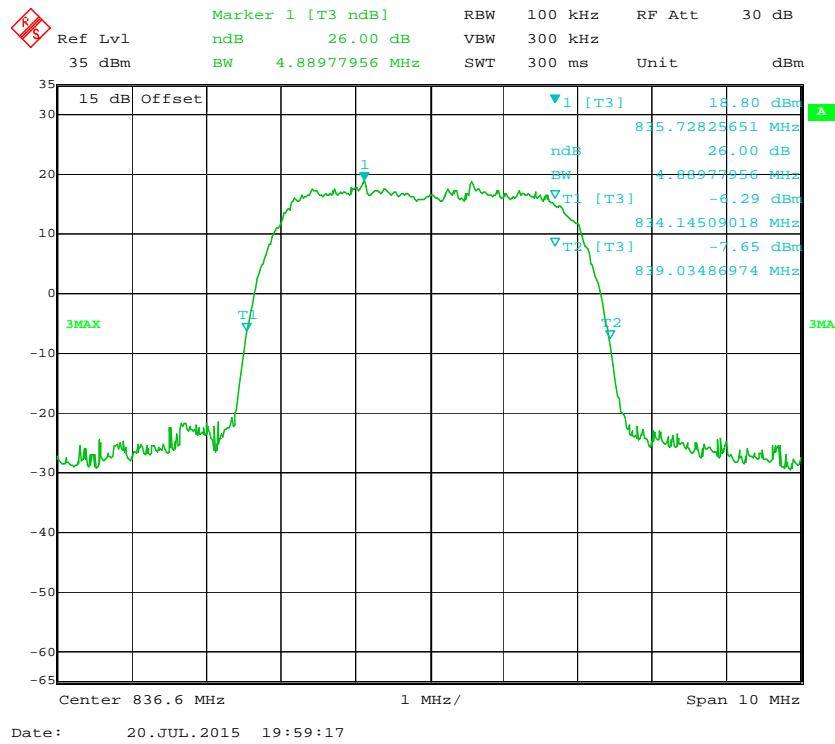
**PCS Band (Part 24E)****99% Occupied Bandwidth for GSM (GMSK) Mode**
