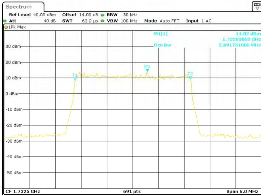
**16-QAM (3.0 MHz) - 99% Occupied Bandwidth, Middle channel**
