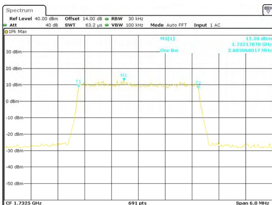
**QPSK (5.0 MHz) - 99% Occupied Bandwidth, Middle channel**
