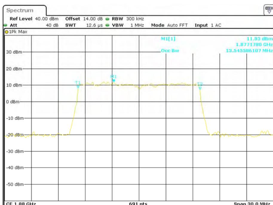
**QPSK (20.0 MHz) - 99% Occupied Bandwidth, Middle channel**
