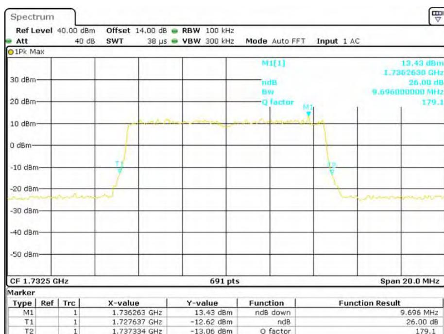
**QPSK (15.0 MHz) - 26 dB Bandwidth, Middle channel**
