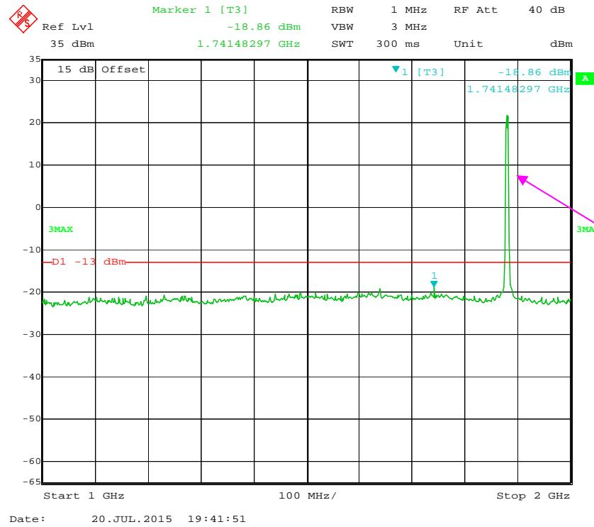
Fundamental test with notch filter
