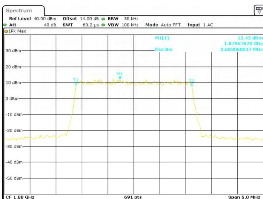
**QPSK (5.0 MHz) - 99% Occupied Bandwidth, Middle channel**
