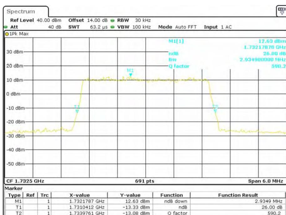
**QPSK (5.0 MHz) - 26 dB Bandwidth, Middle channel**
