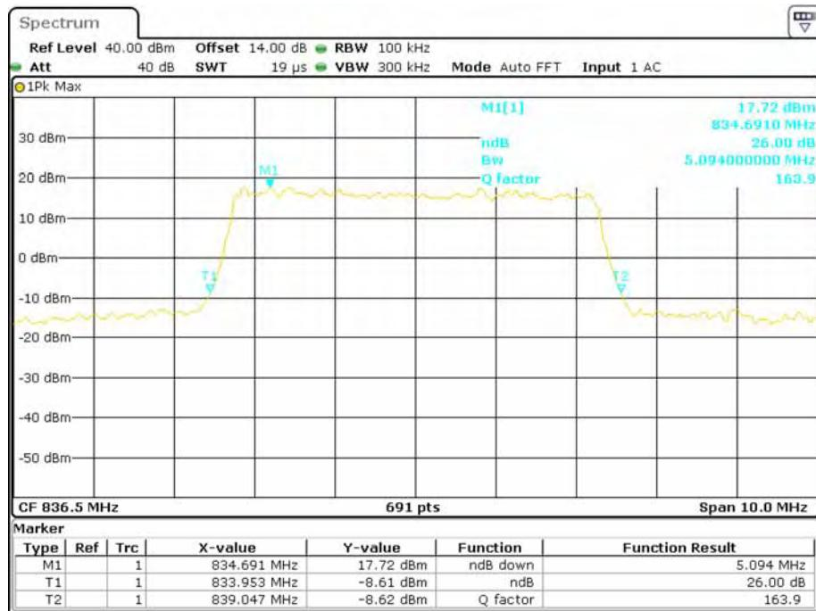
**16-QAM (5.0 MHz) - 26 dB Bandwidth, Middle channel**
