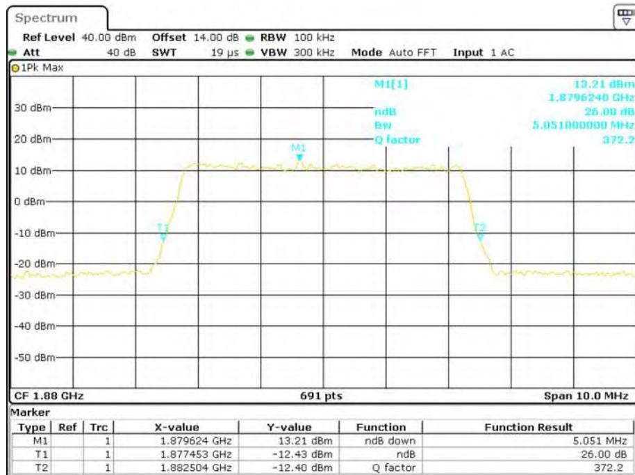
**QPSK (10.0 MHz) - 26 dB Bandwidth, Middle channel**
