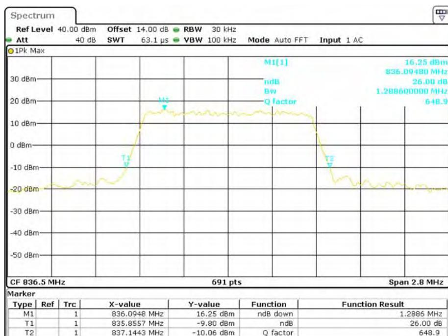
**QPSK (3.0 MHz) - 26 dB Bandwidth, Middle channel**
