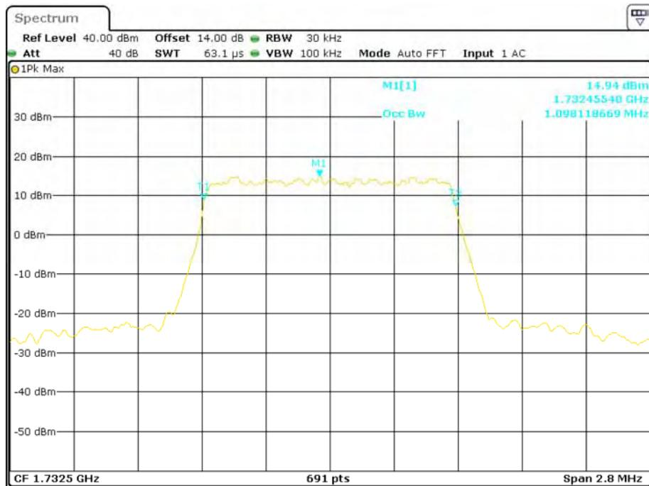
**16-QAM (1.4 MHz) - 99% Occupied Bandwidth, Middle channel**
