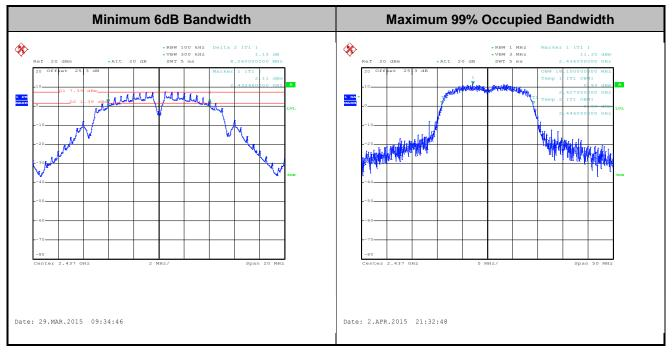
Note: The occupied channel bandwidth is maintained within the band of operation for all of the modulations.
