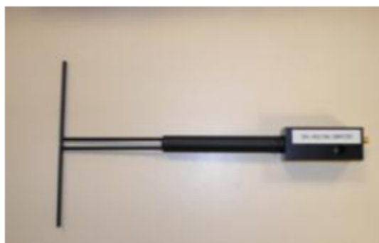
Figure 1 – Satimo COMOSAR Validation Dipole
