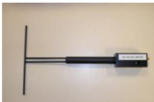
Figure 1 – Satimo COMOSAR Validation Dipole
