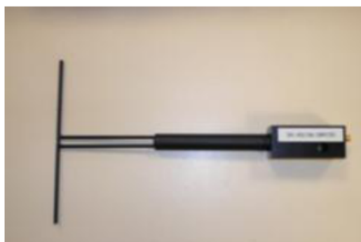
Figure 1 – Satimo COMOSAR Validation Dipole
