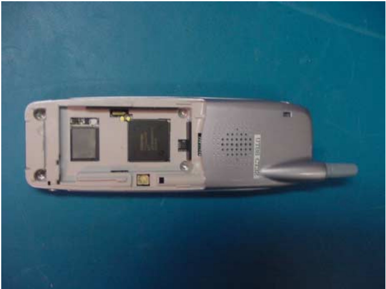
PHOTOGRAPH 19: REAR WITH BATTERY REMOVED
