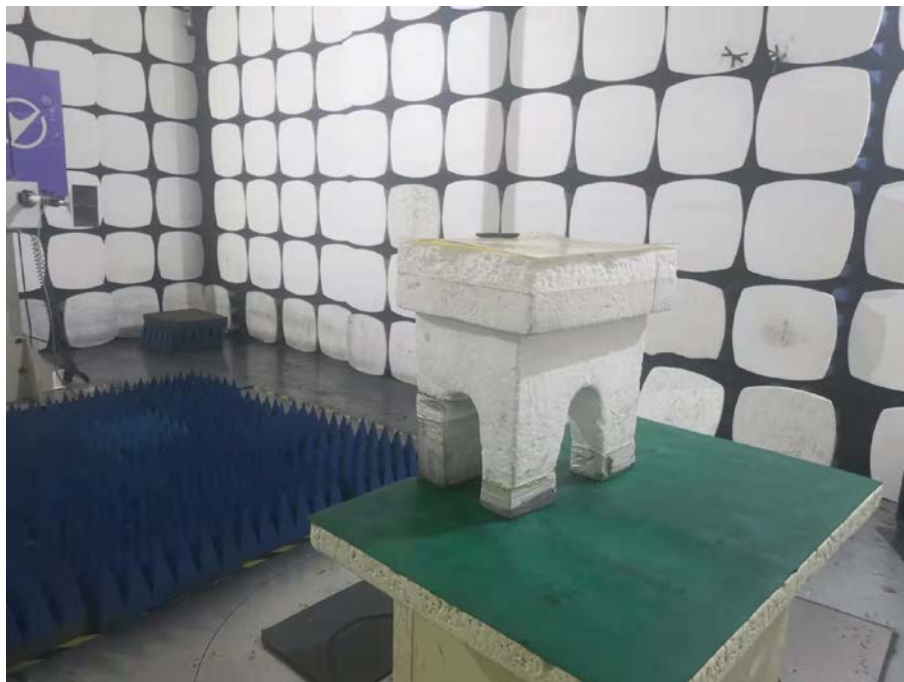
Spurious Emission Test Setup (Above 1GHz)
