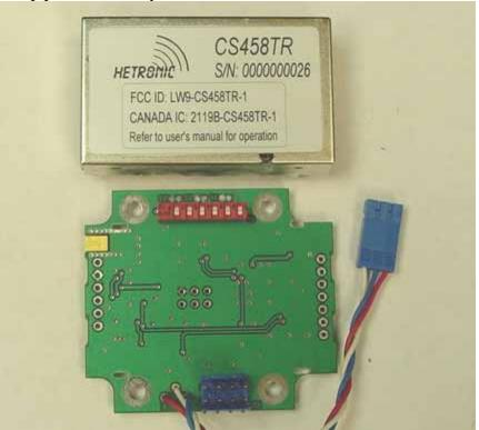
2. Synthesizer top parts (cover removed).
