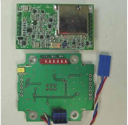
3. Synthesizer top parts (shield removed)
