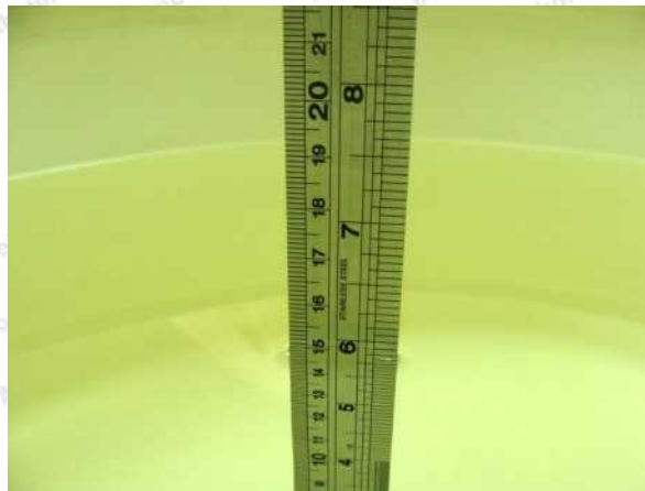
Photo of Liquid Height for Body SAR
