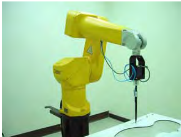
Fig. 5.2 Probe setup on robot
