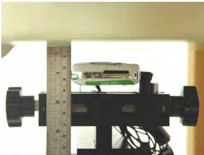
Fig. 9.7 Keypad Up with 1.5cm Gap
