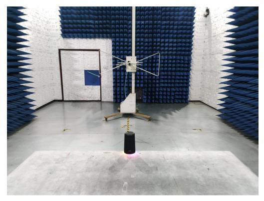
RADIATED EMISSION TEST SETUP ABOVE 1GHz
