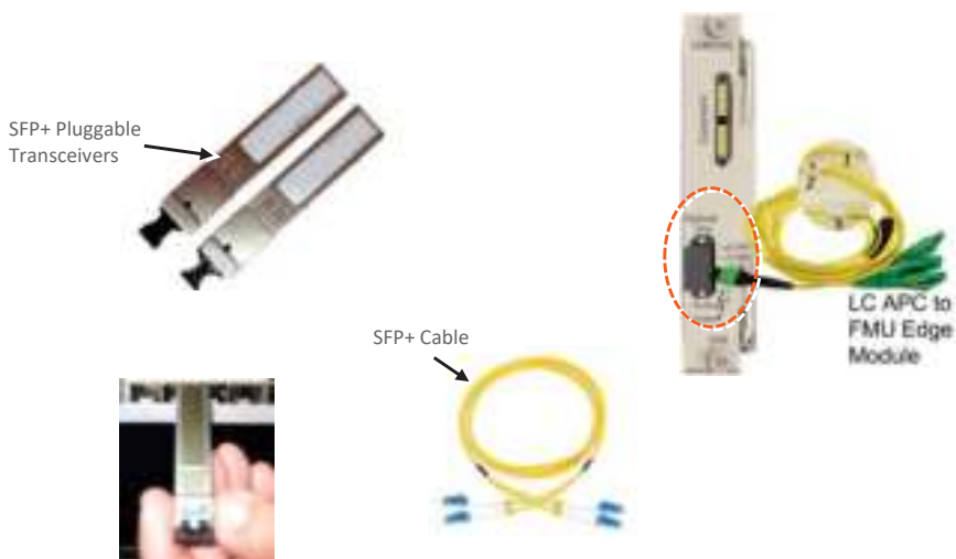
Figure 6 OIM SFP+ LC/UPC connection: Remove rubber stopper from port and from SFP+ Pluggable Transceiver and insert the SFP+ Pluggable Transceivers (hot-pluggable optical transceiver module) into the port.
