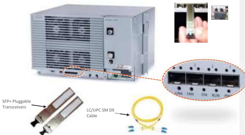
Figure 15 Remove rubber stopper from port and from SFP+ Pluggable Transceiver and insert the SFP+ Pluggable Transceivers (hot-pluggable optical transceiver module) into the port.
