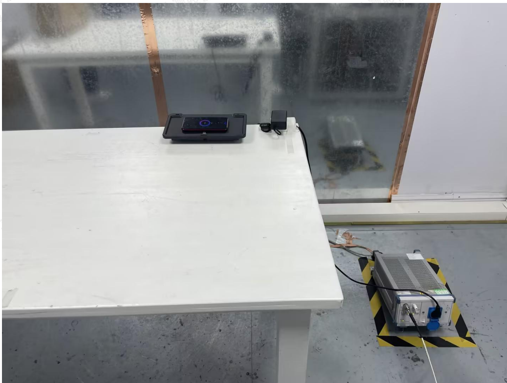
Conducted Emission-AC adapter charge mode
