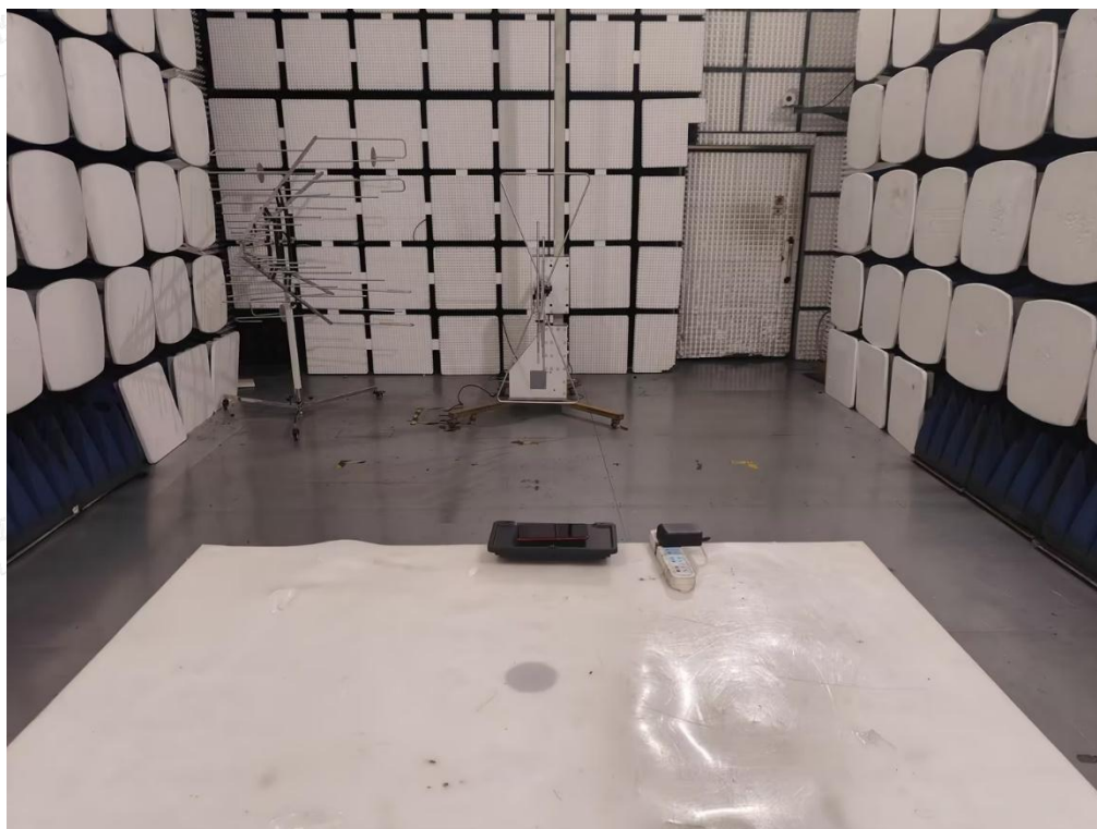
Radiated Emission below 1GHz-AC adapter charge mode
