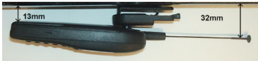
Picture 2. Separation distance with Belt Clip BCH-12U
