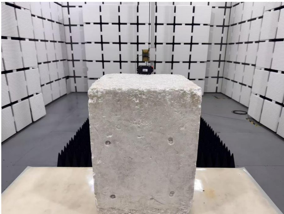
Set-up for Radiated Spurious Emission, Above 1GHz
