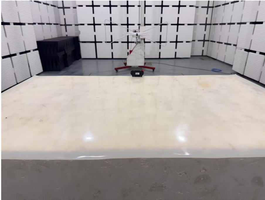
Set-up for Radiated Spurious Emission, Above 1GHz
