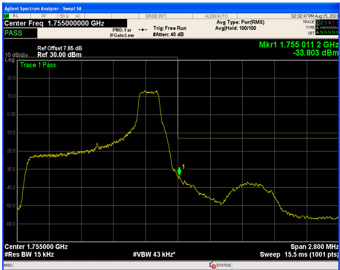
Band4 QPSK BW=1.4MHz Channel=20393 RB Size=6 Position=#0
