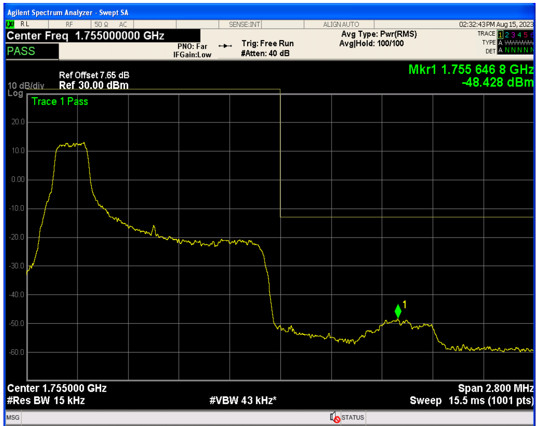
Band4 QPSK BW=1.4MHz Channel=20393 RB Size=1 Position=#Max
