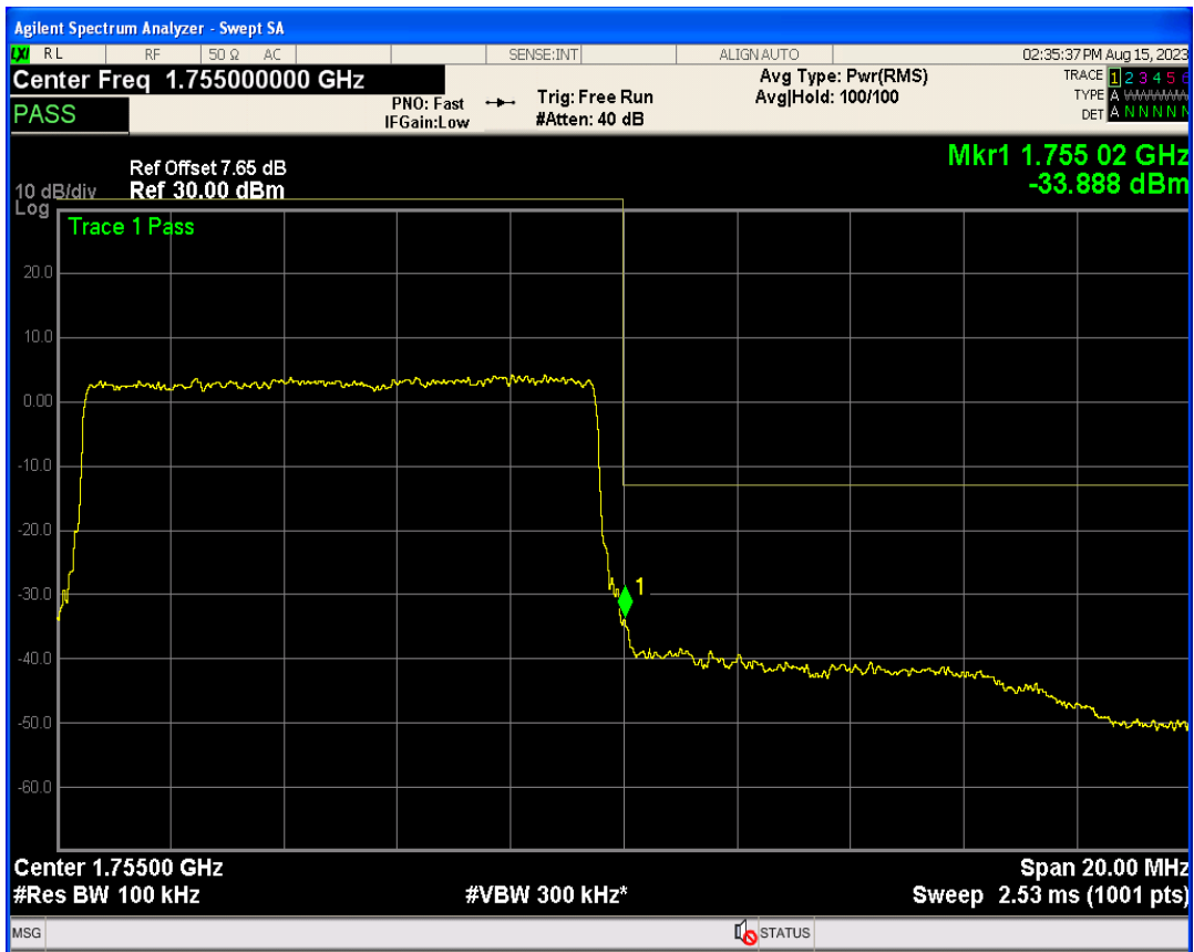
Band4 16QAM BW=10MHz Channel=20350 RB Size=1 Position=#0
