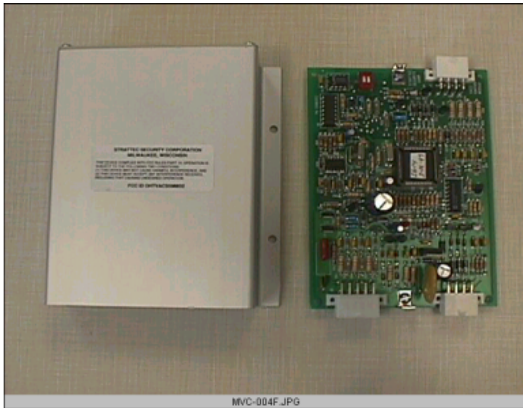
Strattec - Ignition Module PCB open for inspection
