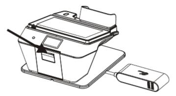
2) Load the paper roll into the paper compartment in the direction displayed on the back of the cover into the paper compartment and extend the end of the paper out of printer.
