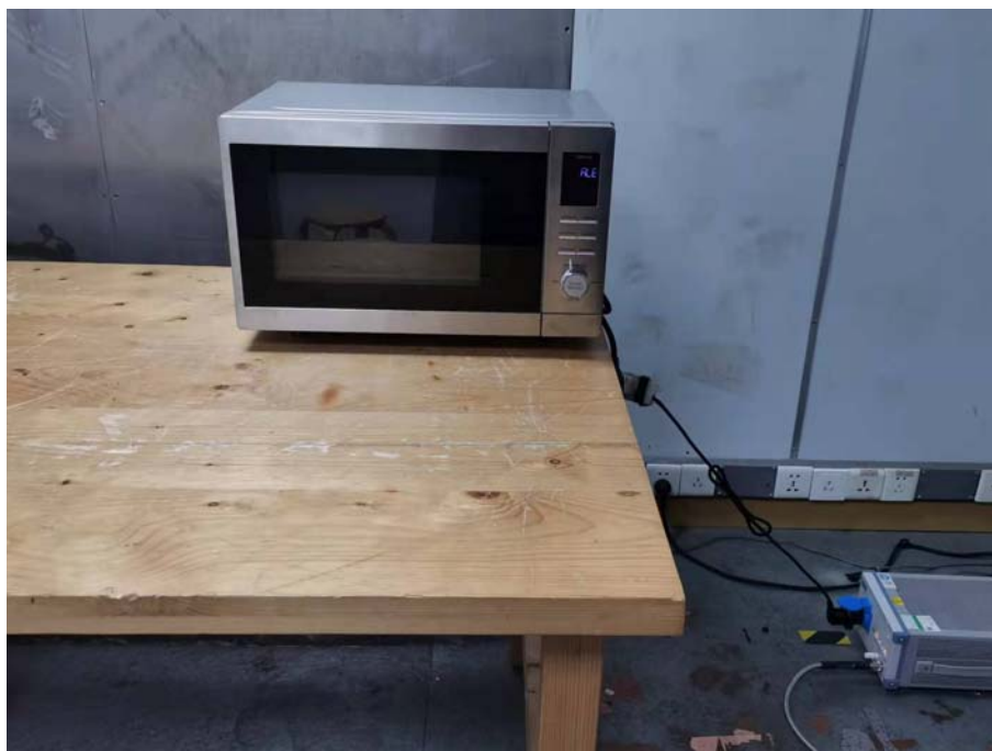
Photo of Power Line Conducted Emission Measurement
