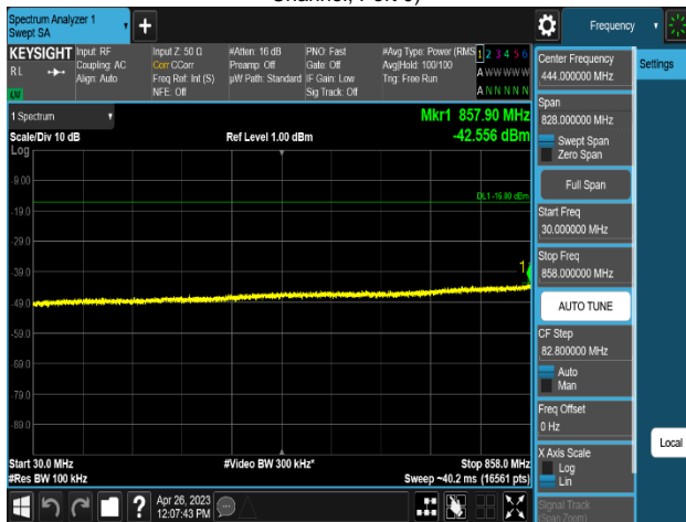
Plot 8-551. Conducted Spurious Emission Plot 30 MHz to 858 MHz (MSR 2NC_DSS B(n)5_1C_10M+NR n5_1C_5M_2T_QPSK-Middle Channel, Port 0)
