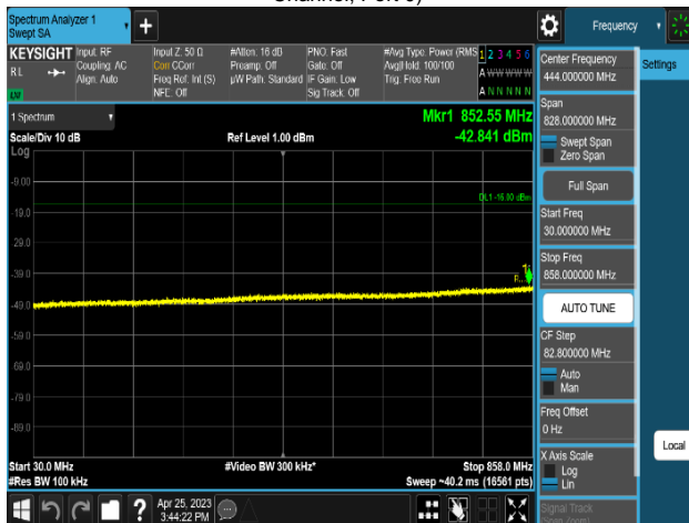
Plot 8-527. Conducted Spurious Emission Plot 30 MHz to 858 MHz (MSR 3C_NR n5_2C_10M+10M+LTE B5_1C_5M_2T_QPSK-Mid Channel, Port 0)
