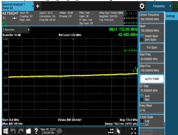
Plot 8-575. Conducted Spurious Emission Plot 30 MHz to 735 MHz (LTE B13_1C_5M_2T_256QAM - High Channel, Port 1)
