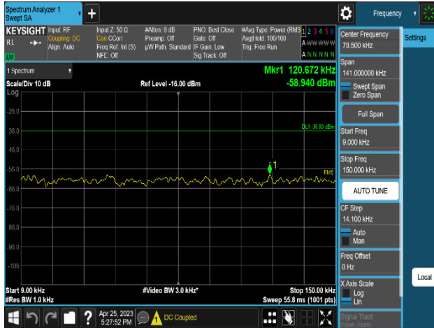
Plot 8-543. Conducted Spurious Emission Plot 9 kHz to 150 kHz (MSR 2C_DSS B(n)5_1C_10M+NR n5_1C_15M_2T_16QAM-Low Channel, Port 0)
