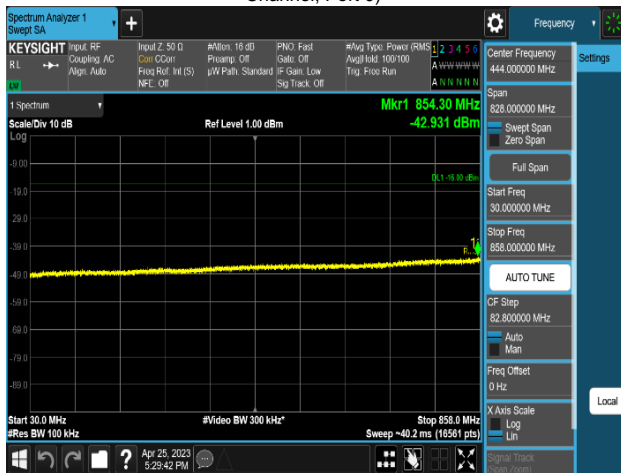
Plot 8-545. Conducted Spurious Emission Plot 30 MHz to 858 MHz (MSR 2C_DSS B(n)5_1C_10M+NR n5_1C_15M_2T_16QAM-Low Channel, Port 0)
