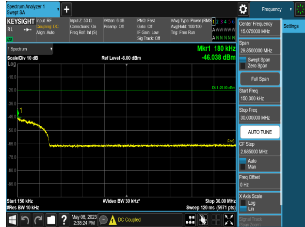
Plot 8-574. Conducted Spurious Emission Plot 150 kHz to 30 MHz (LTE B13_1C_5M_2T_256QAM - High Channel, Port 1)
