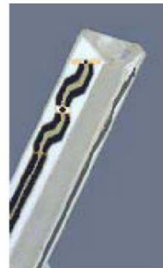
Figure 2.3 Probe Thick-Film Technique
