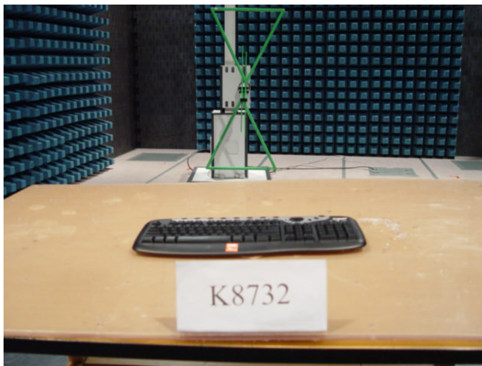
Photograph 2: Set-up for Radiation Measurement below 1GHz
