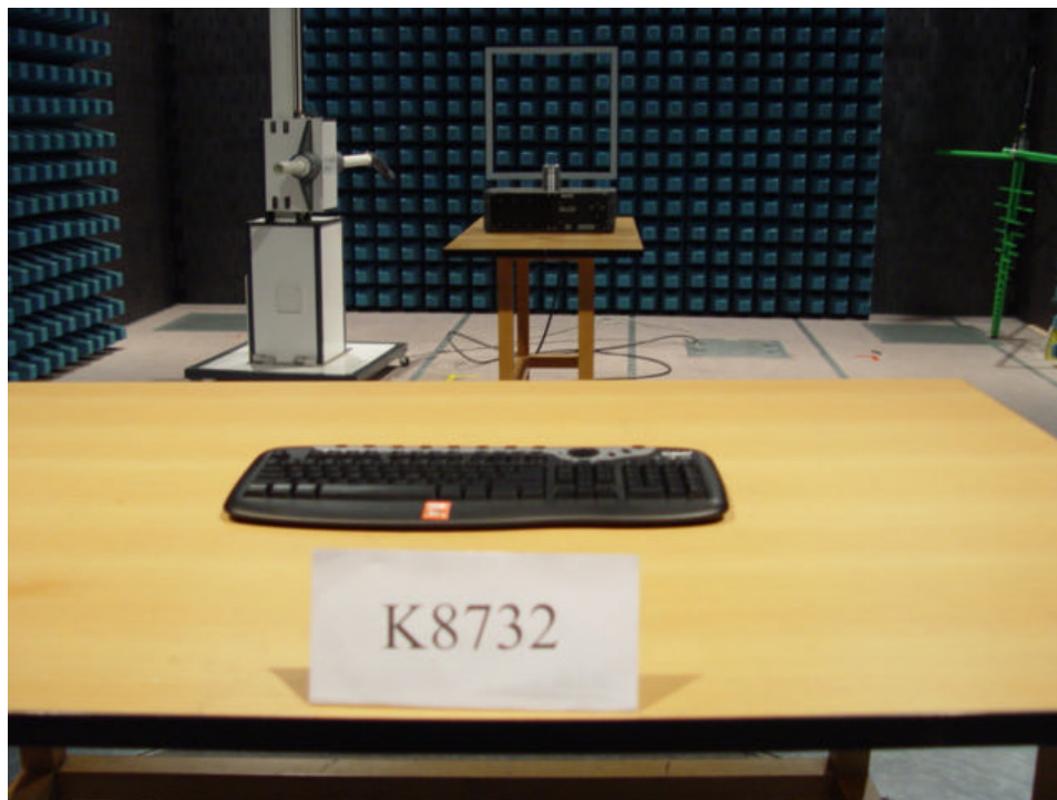
Photograph 1: Set-up for Radiation Measurement Below 30MHz
