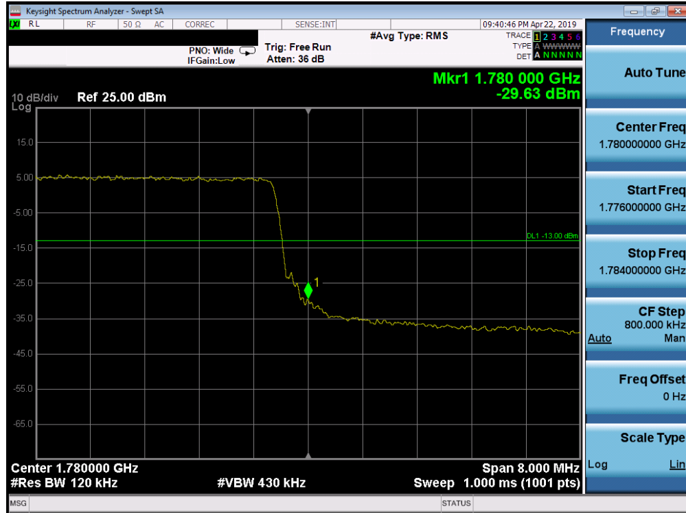
Plot 7-213. Upper Band Edge Plot (Band 66 - 10.0MHz QPSK - Full RB Configuration)
