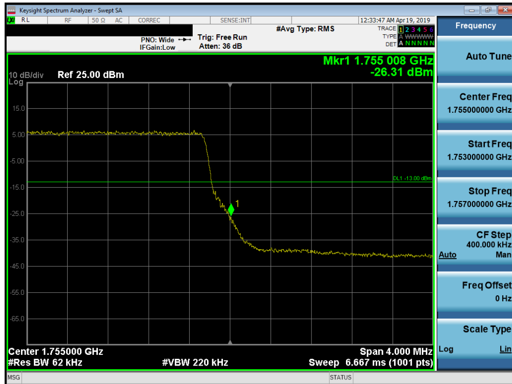
Plot 7-205. Upper Band Edge Plot (Band 4 – 5.0MHz QPSK - Full RB Configuration)
