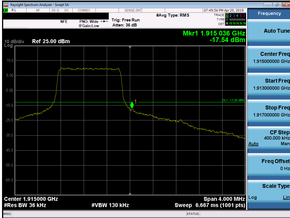
Plot 7-231. Upper Band Edge Plot (Band 25 - 1.4MHz QPSK - Full RB Configuration)
