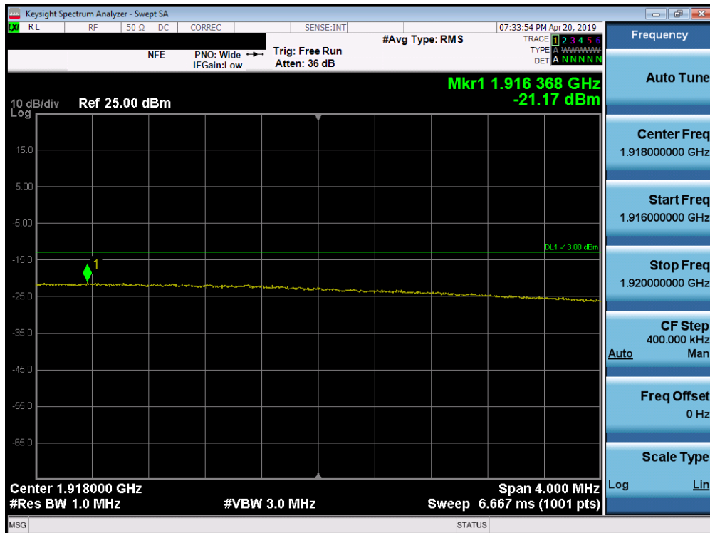
Plot 7-256. Upper Extended Band Edge Plot (Band 25 - 15.0MHz QPSK - Full RB Configuration)
