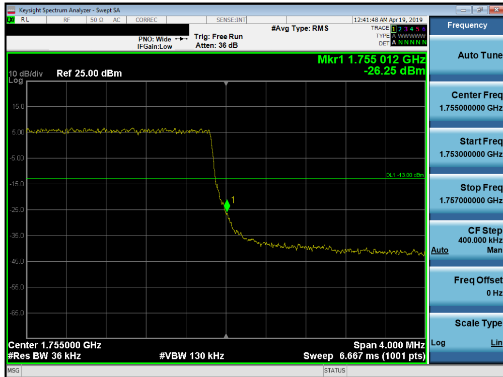
Plot 7-199. Upper Band Edge Plot (Band 4 – 3.0MHz QPSK - Full RB Configuration)
