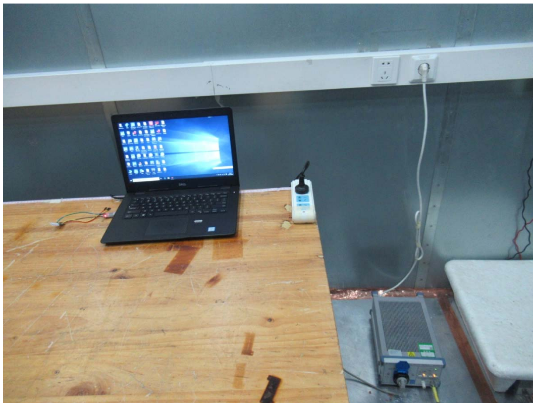
Picture 1: Conducted Emissions Test Setup
