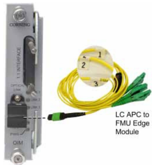
Figure 4-21. OIM Fiber Connections
