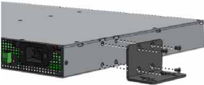
Figure 5-4. DC Assembling Wall Mount Brackets
