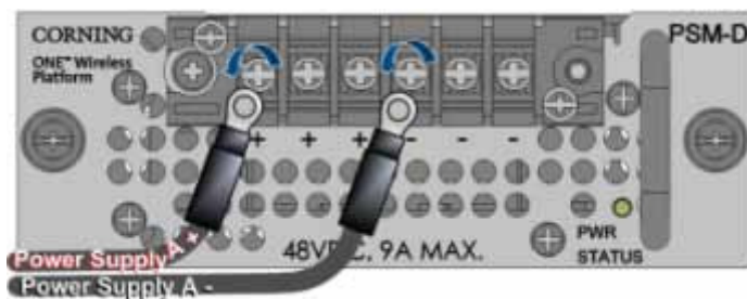
Figure 4-26. Connecting PSM-DC Wire Pairs
