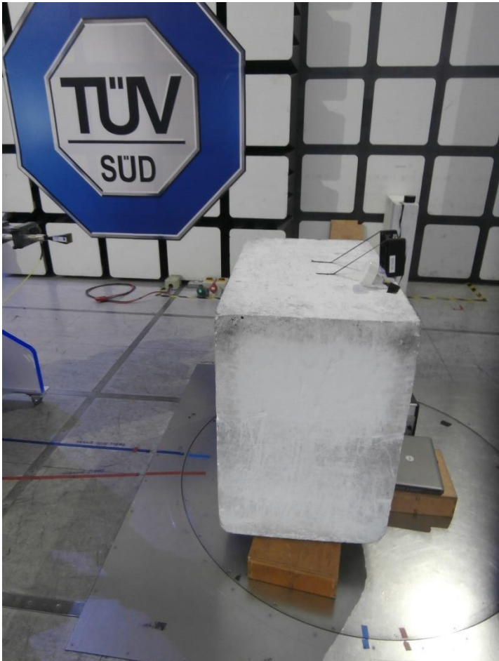
Figure 7 – Test Setup 18 GHz to 30 GHz - Y Orientation
