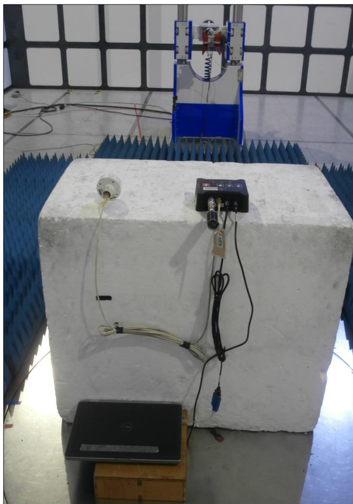
Figure 25 - Test Setup 1 GHz to 18 GHz - X Orientation
