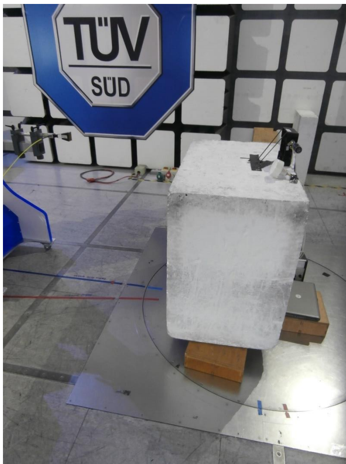
Figure 8 – Test Setup 18 GHz to 30 GHz - Z Orientation
