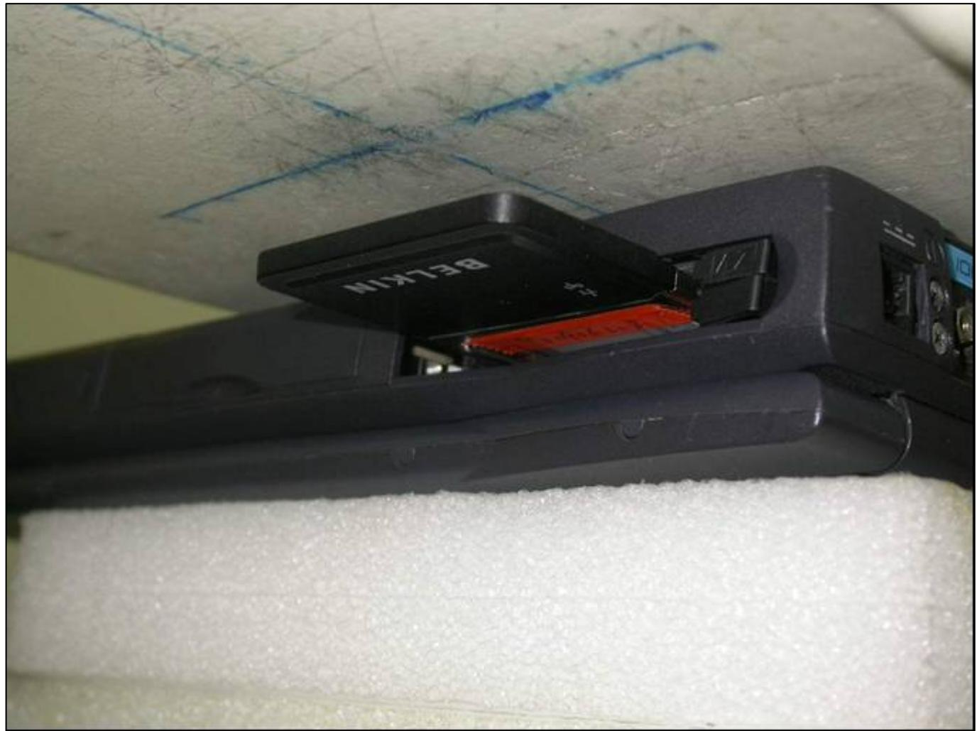
The bottom of the EUT to the flat phantom distance 11 mm
