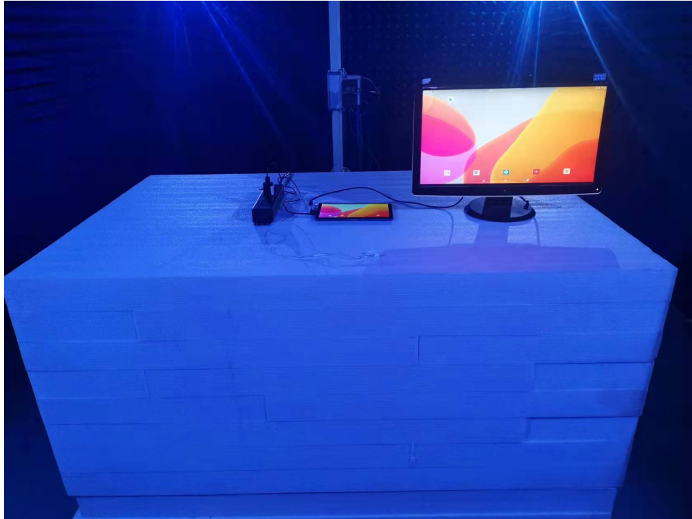
Photo of Radiated Emission Measurement (Above 1G)
