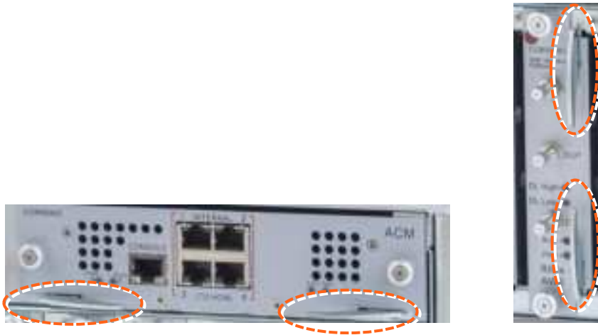
Figure 13: Module Captive Screws and Ejectors
