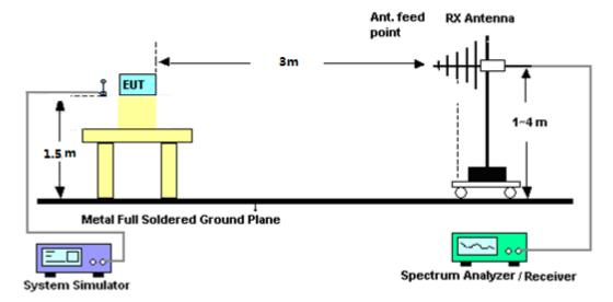
For radiated test from above 1GHz
