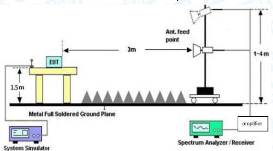
**Above 1GHz Test Setup**
