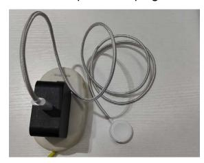
2. Put the apple watch on the module side of the product, The center of the watch is aligned with the center of the module, If the watch displays the green lightning icon, it is normally charged
