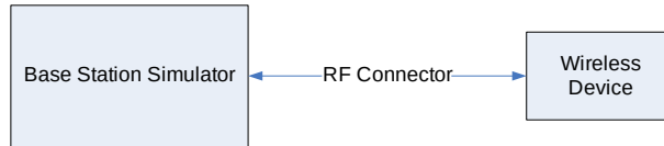
Figure 8-1 Power Measurement Setup
