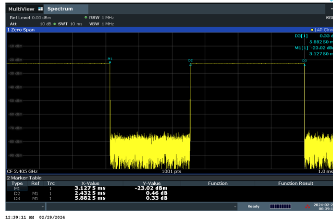
Equation 8-6 802.15.4 Duty Cycle Calculation – Antenna 4a/2a, Variant 2
