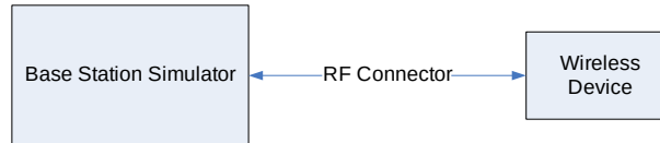
Figure 8-2 Power Measurement Setup
